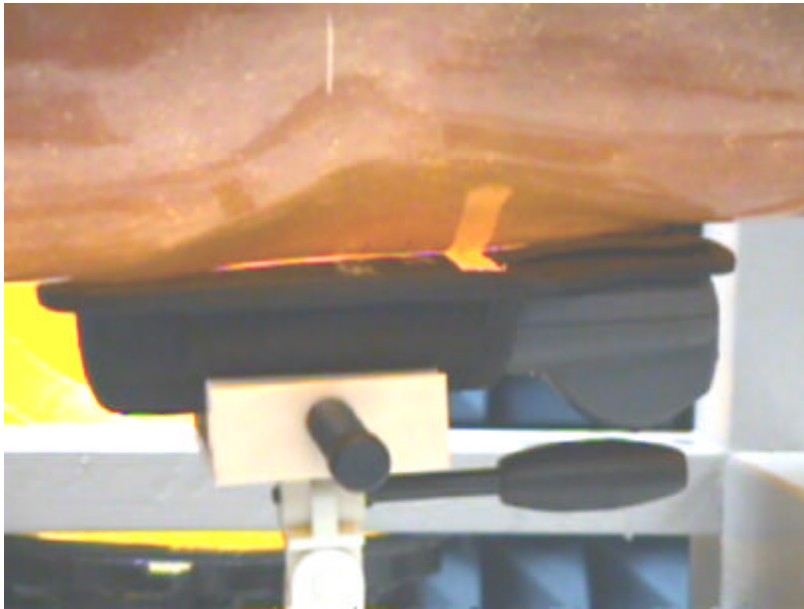
Figure 1: Hand-held data terminal (HDT515) and FLN9623A holster. Distance from the phantom to the HDT515 = 5.0 mm (Holster is 5.0 mm thick)
