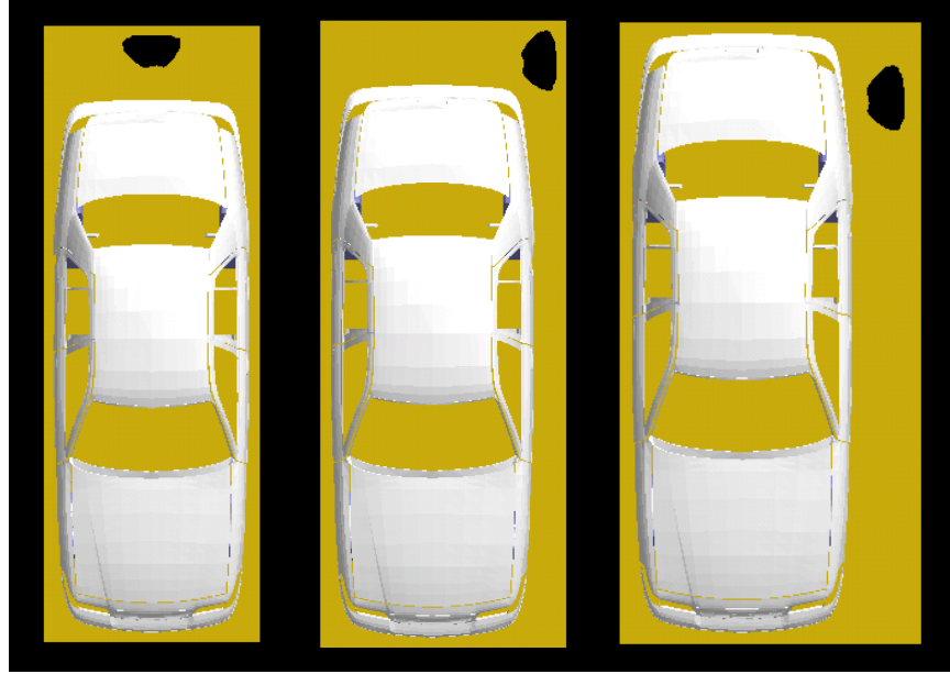
Figure 2: Top view of bystander exposure model four different locations relative to the vehicle model that replicate the measurement conditions.
