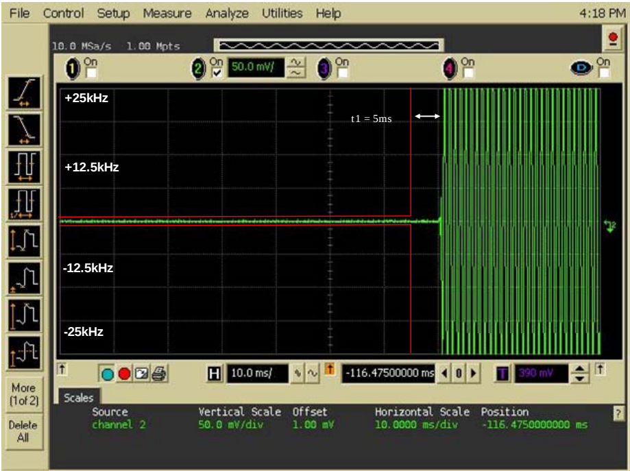
Figure 6I-1: Transient Frequency Behavior. 155.0125 MHz, 25 kHz Channel Spacing, Key-up Transient
