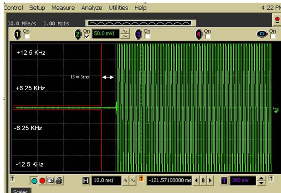
Figure 6I-4: Transient Frequency Behavior. 155.0125 MHz, 12.5 kHz Channel Spacing, De-Key Transient
