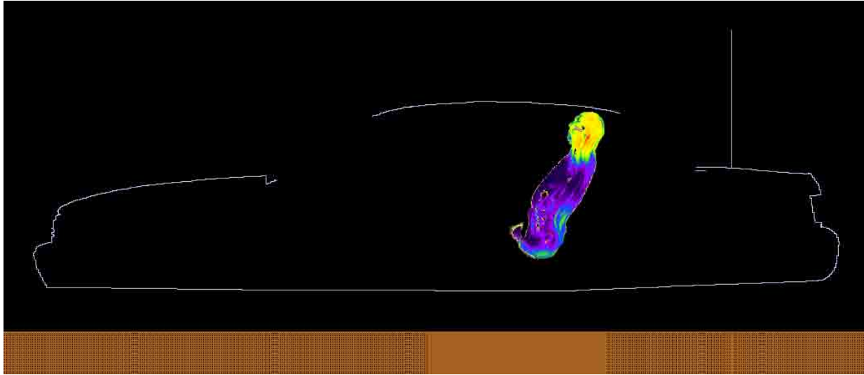
Figure 3. SAR distribution at 173.4 MHz in the passenger model located in the center of the back seat, produced by the trunk-mount HAD4022A antenna. The contour plot is relative to the plane where the peak 1-g average SAR for this exposure condition occurs.
