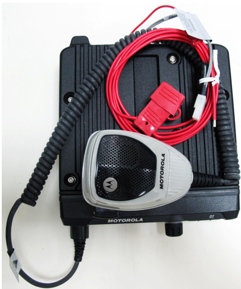
Top view with microphone and rear accessory cable
