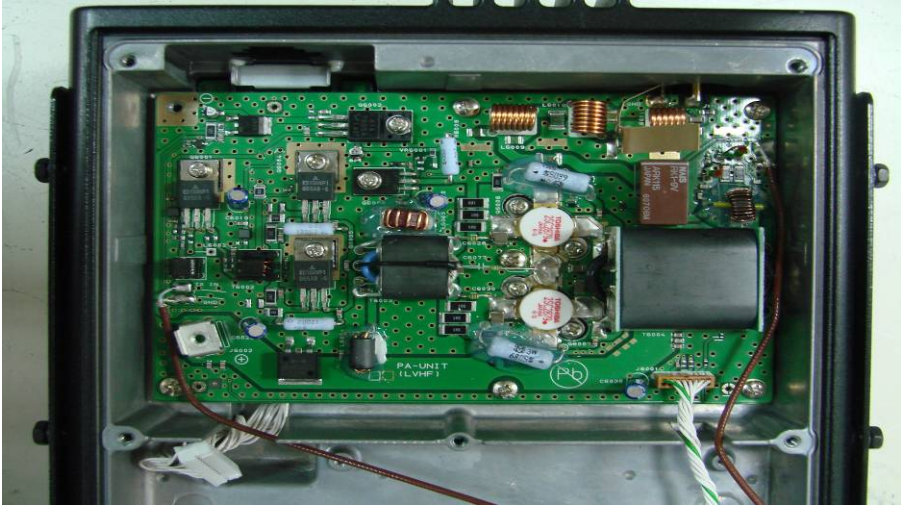
Figure 9.1: RF amplifier unit front view
