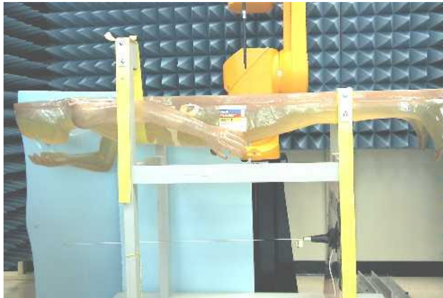
Figure 1 Antenna positioned in front of the phantom man model with the ground plane near knees.
