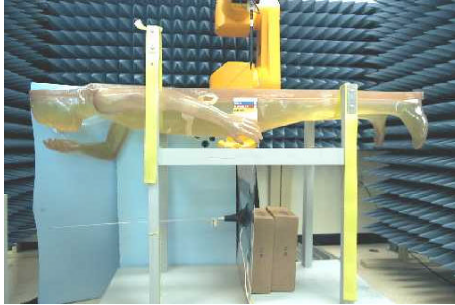
Figure 2 Antenna positioned in front of the phantom man model with the ground plane near abdomen.
