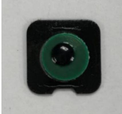
Location of Passive NFC Tag at the Shroud of the LKP Model
