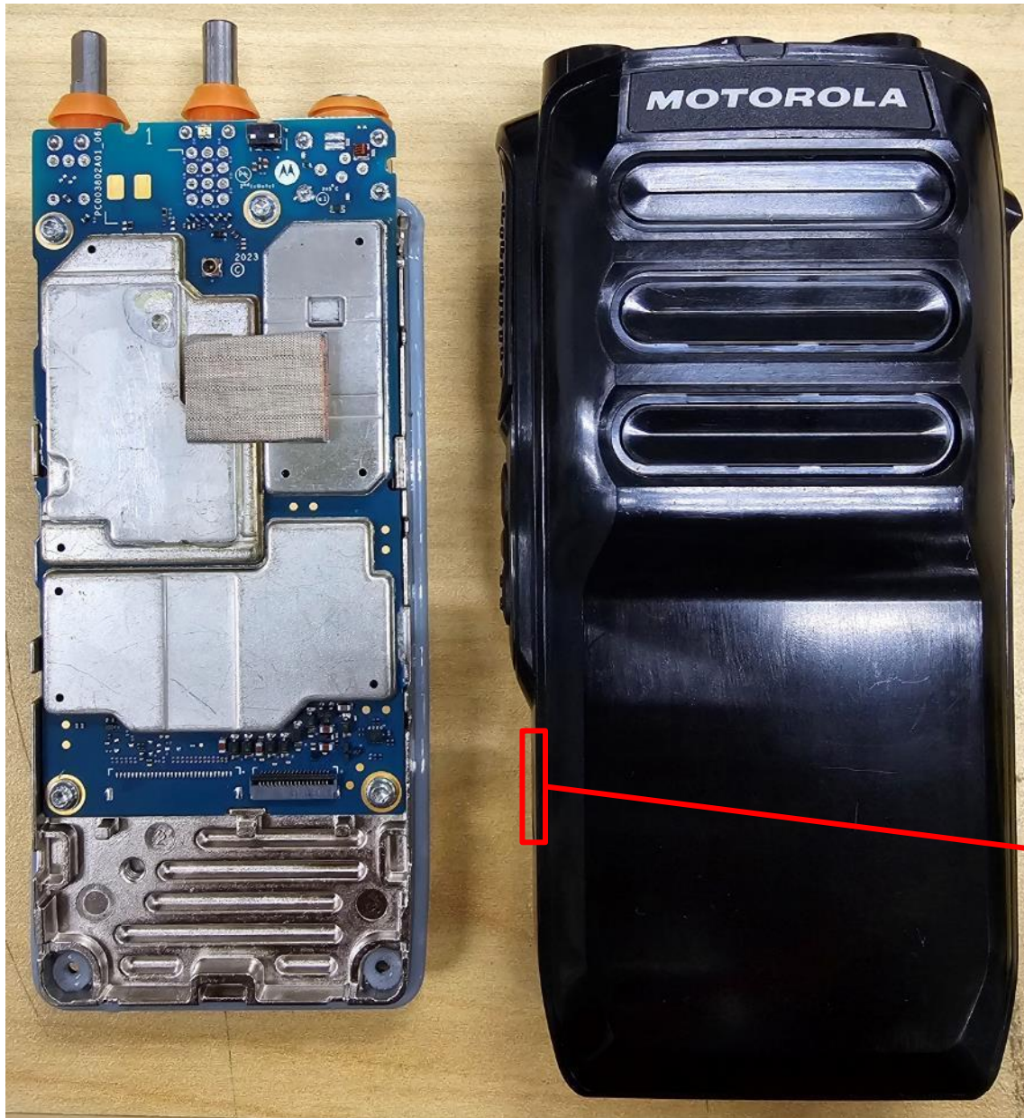
RF boards with chassis and housing for (Front Side) of NKP Model
