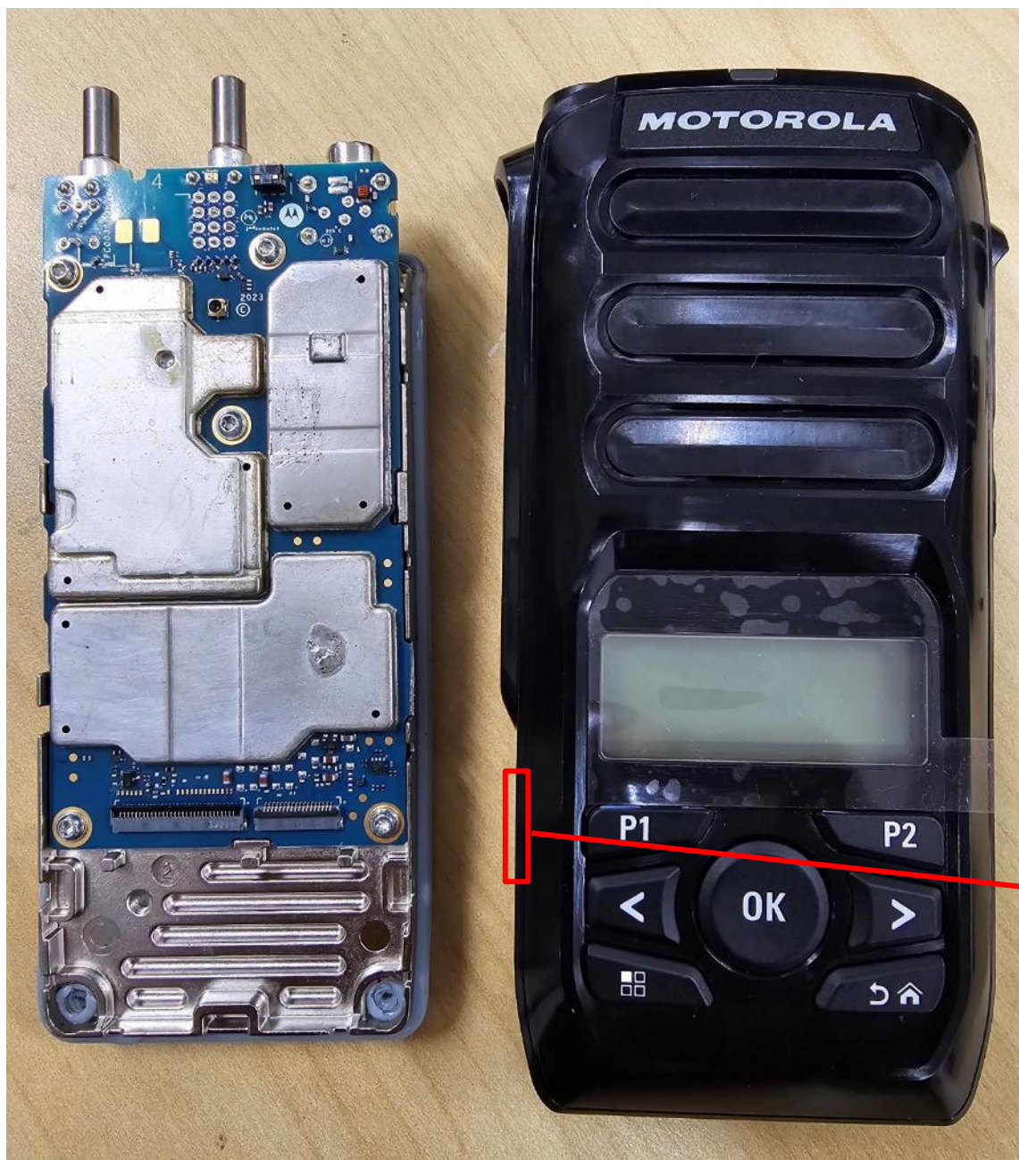
RF boards with chassis and housing for (Front Side) of LKP Model
