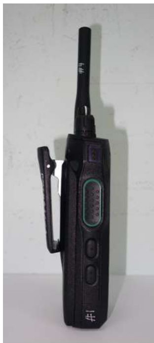
DUT Side View Belt Clip PMLN8369A
