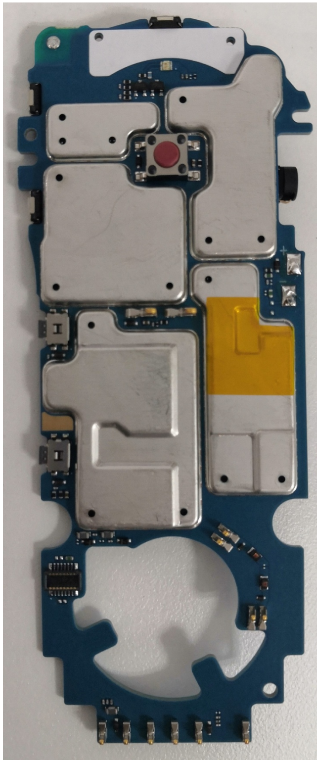
EXHIBIT 9A - RF board with Shields (Top)
