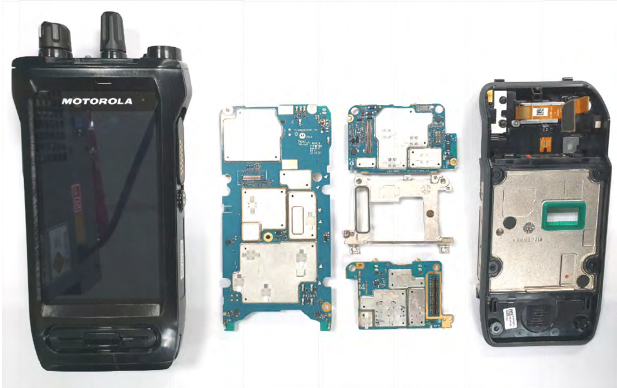
Exhibit 9M: RF boards with chassis and housing for (Front Side)
