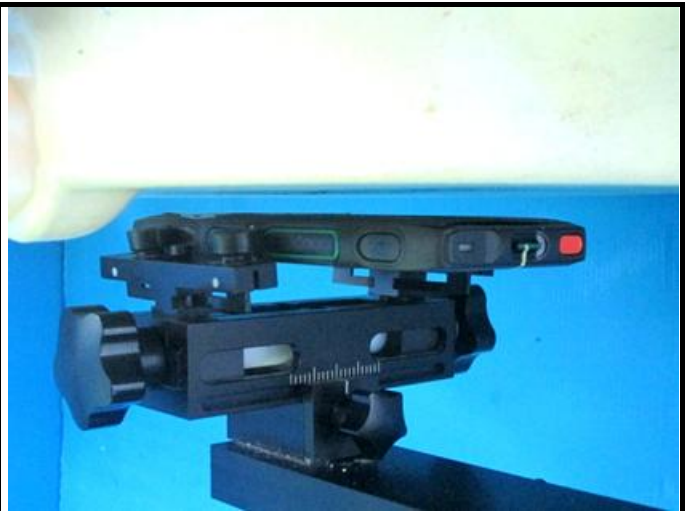
Body - Rear Face of EUT at 10 mm
