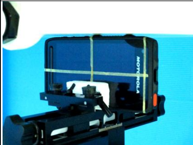
Phablet - Left Side of EUT at 0 mm
