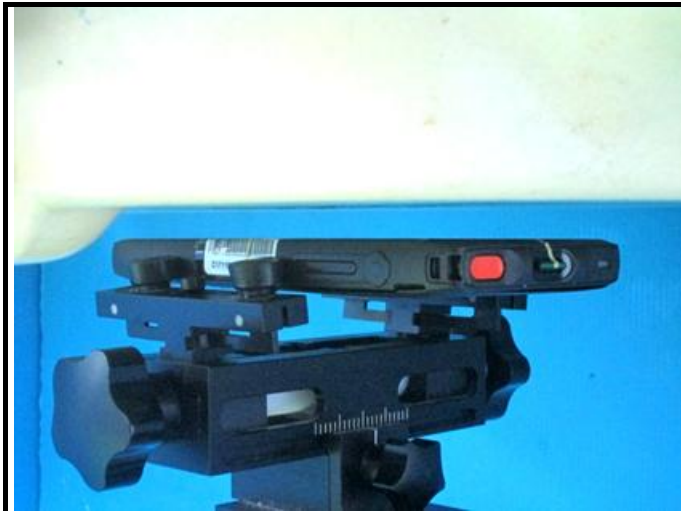
Body - Front Face of EUT at 10 mm
