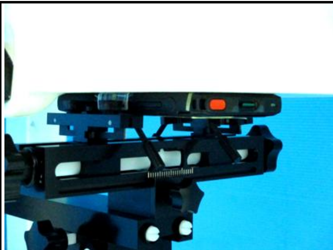
Phablet - Front Face of EUT at 0 mm
