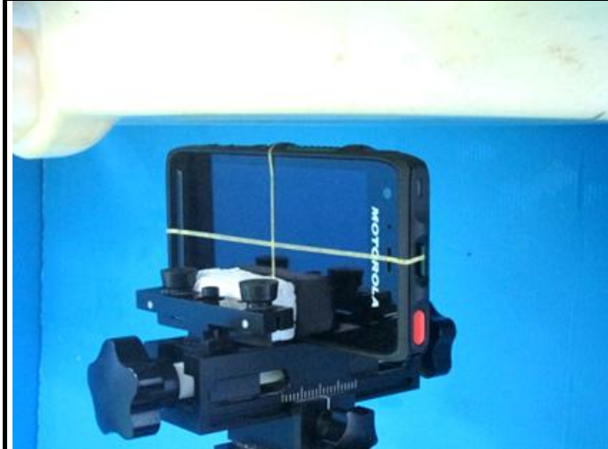
Body - Left Side of EUT at 10 mm
