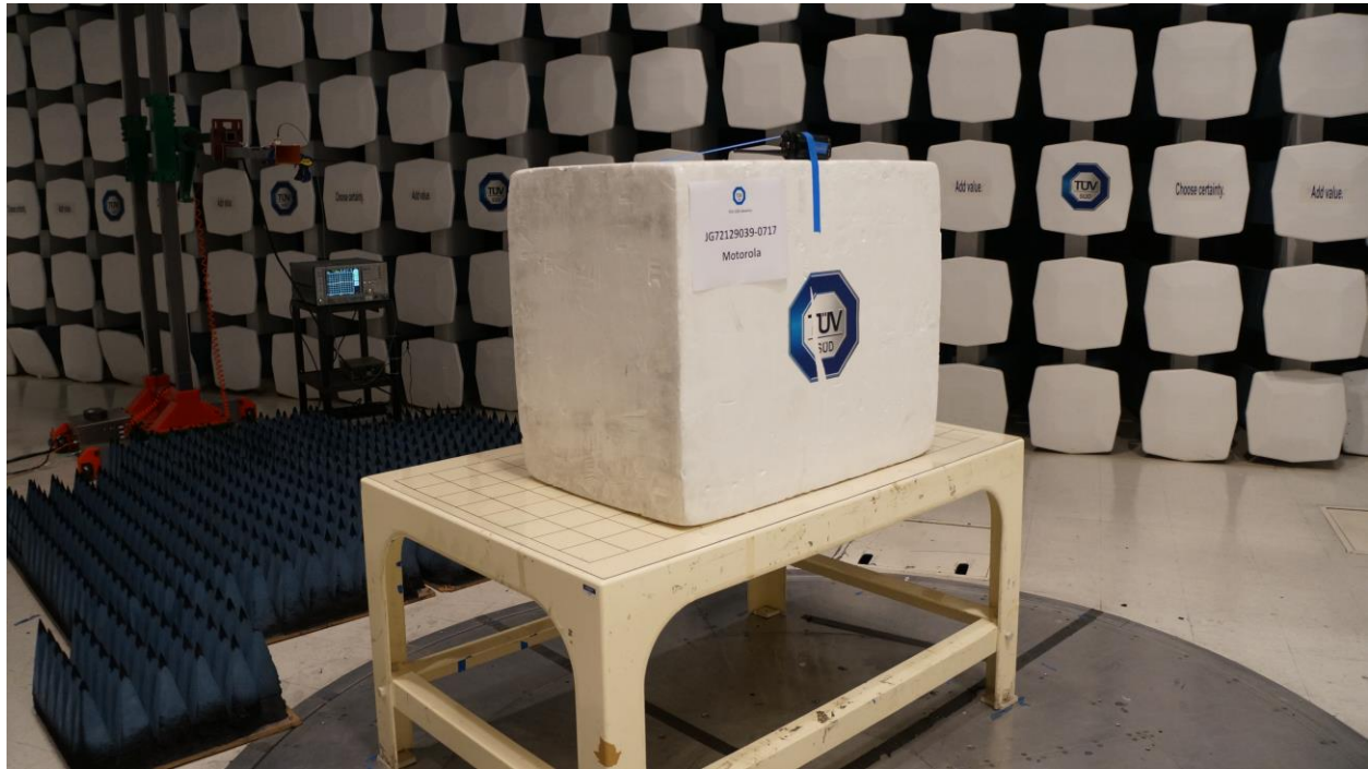
Radiated Emissions Test Setup (Above 18000 MHz - Back)
