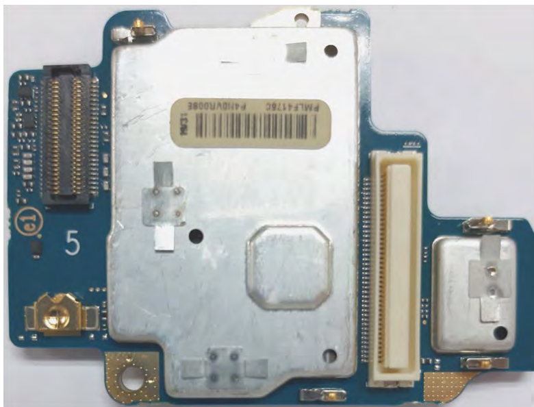
Vocon board with shields (Bottom) (APX6000/APX5000/APX6000XE/APX6000Li/SRX2200)
