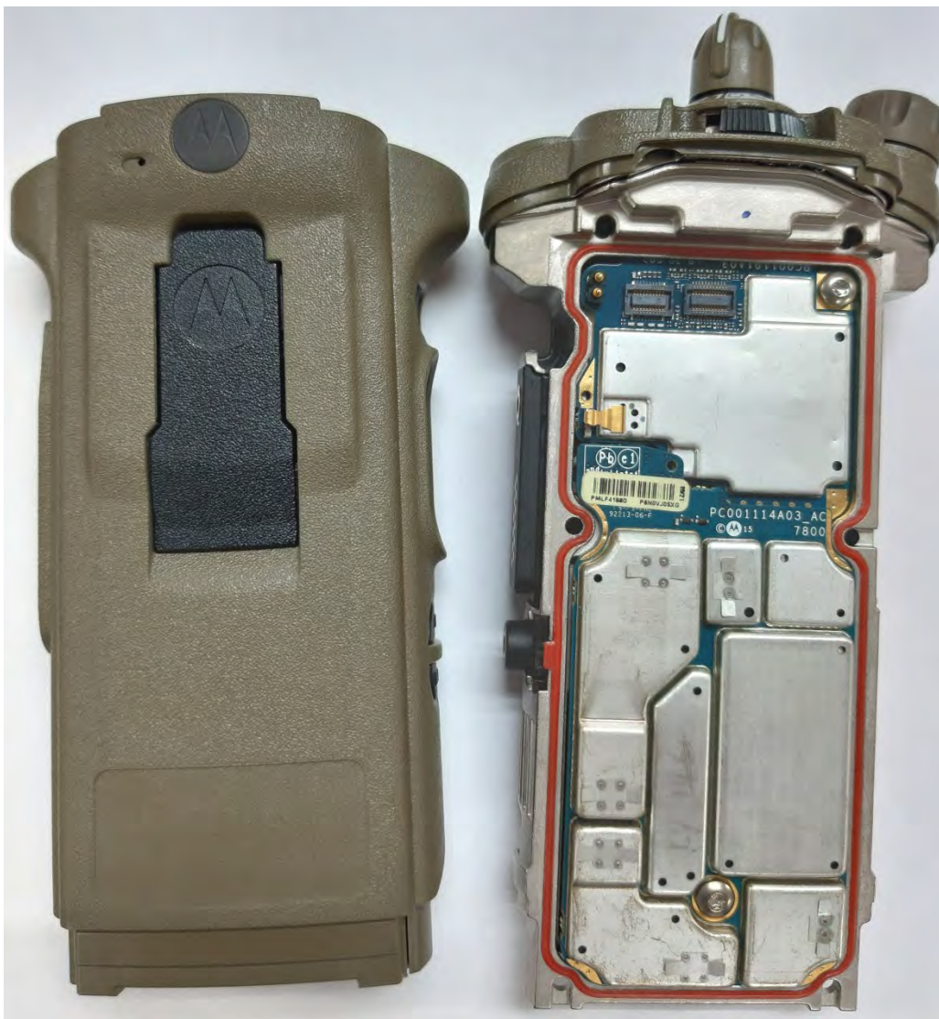
RF and Vocon boards with chassis and housing of SRX2200 Model 1.5 (Front side)
