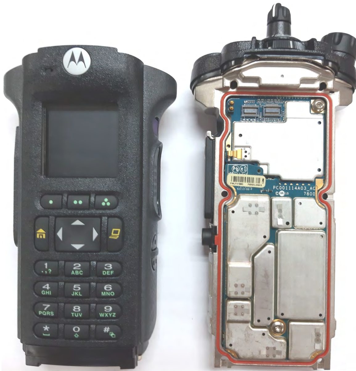
RF and Vocon boards with chassis and housing of APX6000/APX6000Li/APX5000 Model 3.5 (Front side)
