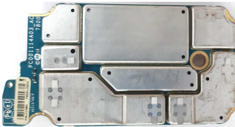
RF board with Shields (Top) (APX6000/APX5000/APX6000XE/APX6000Li/SRX2200)
