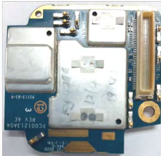
Expansion board with shields (Bottom) (APX6000/APX5000/APX6000XE/APX6000Li/SRX2200)
