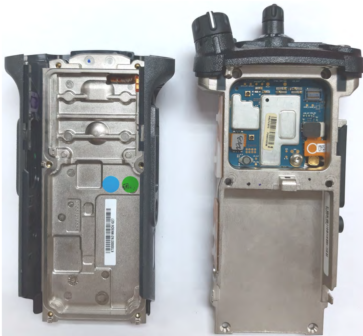
Expansion board with chassis and housing of APX6000/APX6000Li/APX5000 Model 1.5 (Back side)
