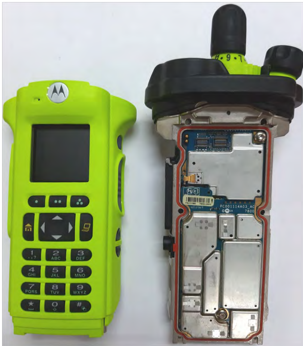
RF and Vocon boards with chassis and housing of APX6000XE Model 3.5 (Front side)
