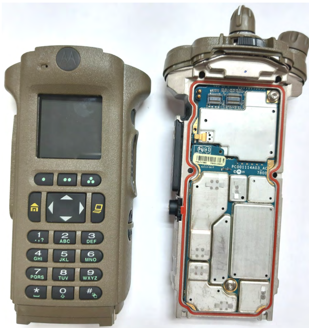
RF and Vocon boards with chassis and housing of SRX2200 Model 3.5 (Front side)
