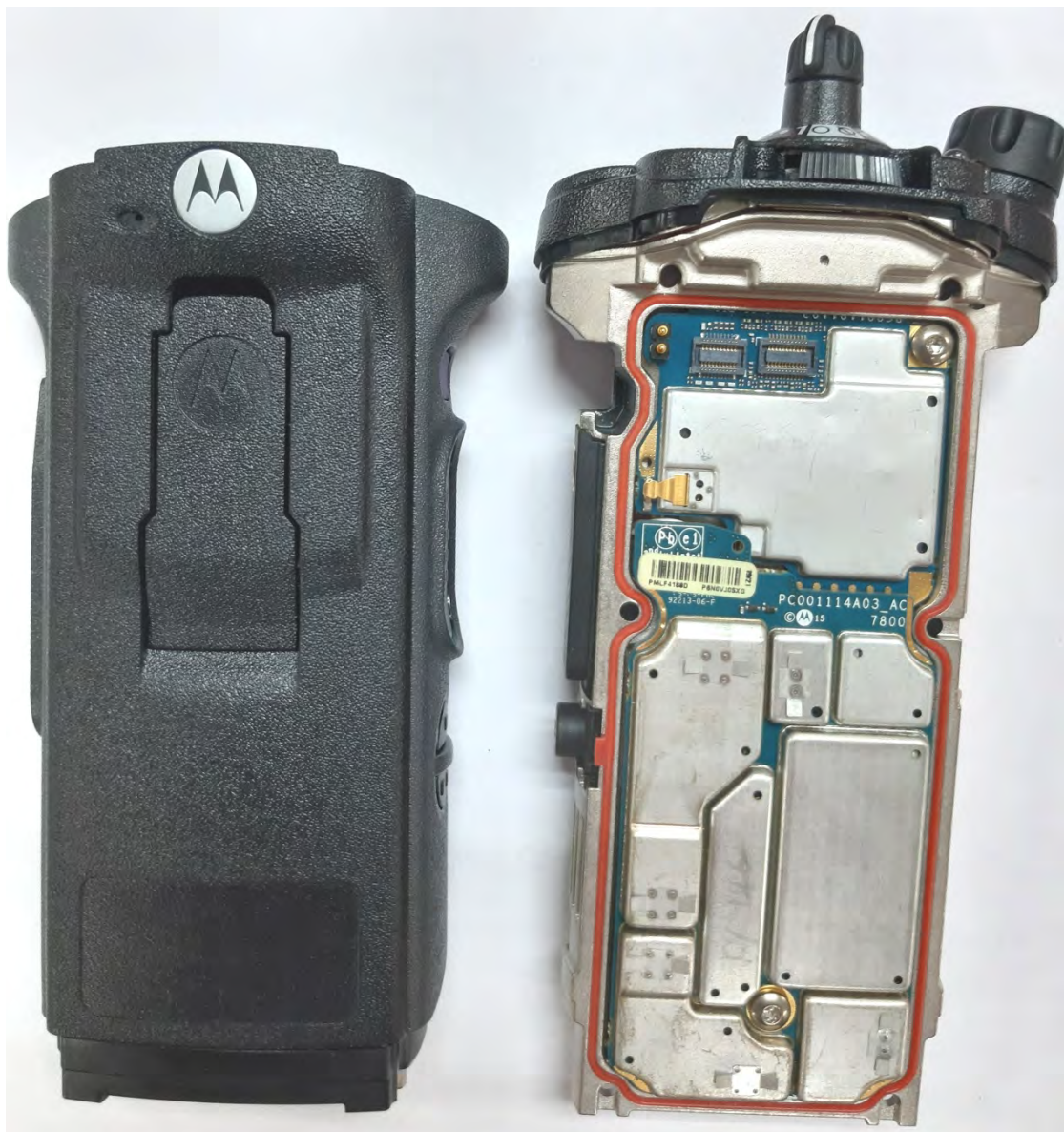
RF and Vocon boards with chassis and housing of APX6000/APX6000Li/APX5000 Model 1.5 (Front side)
