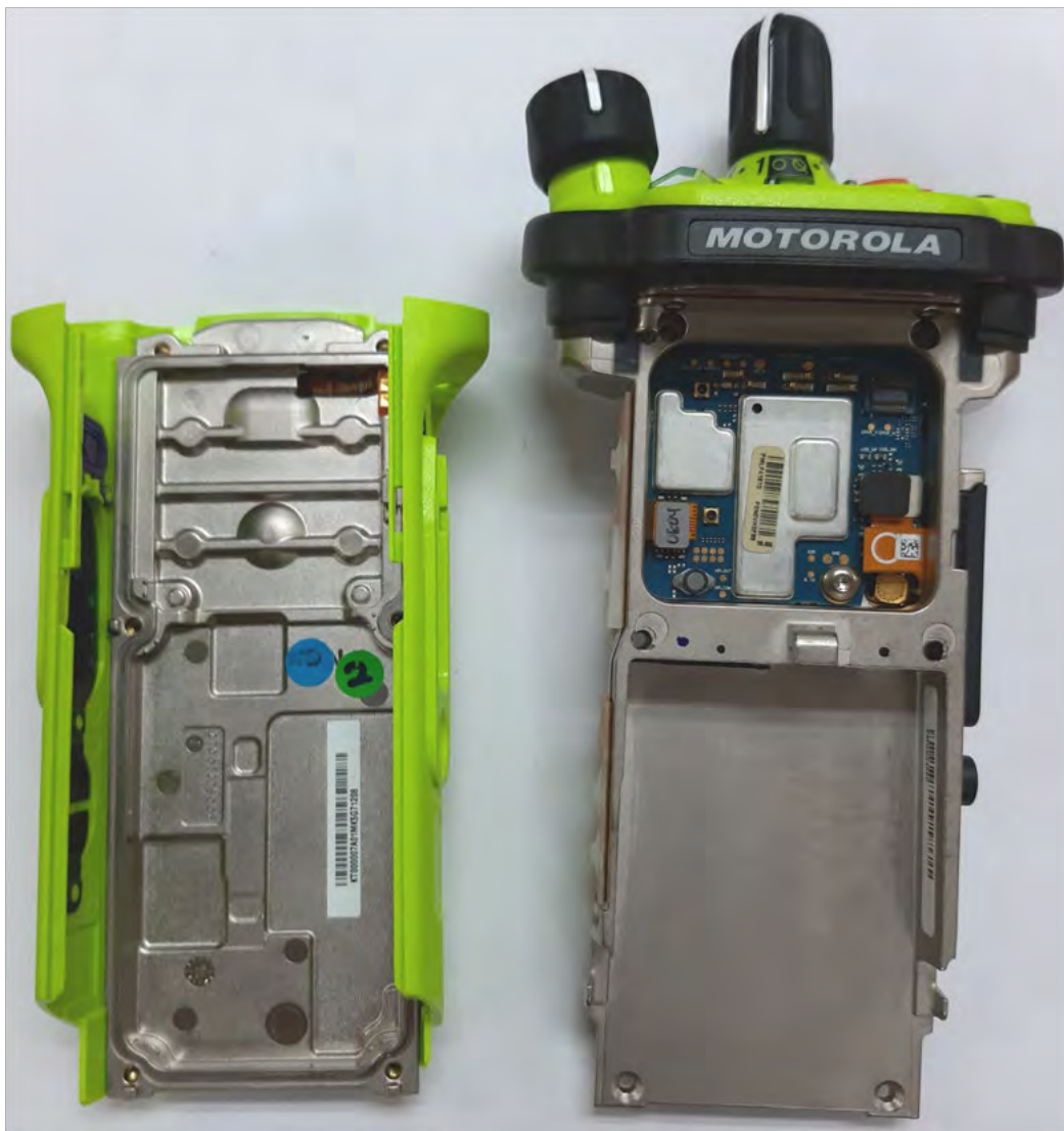
Expansion board with chassis and housing of APX6000XE Model 1.5 (Back side)
