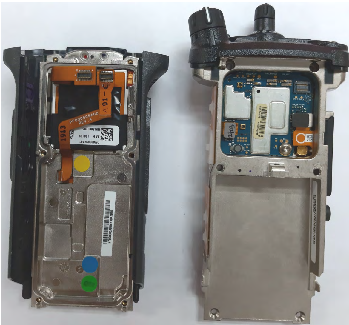
Expansion board with chassis and housing of APX6000/APX6000Li/APX5000 Model 3.5 (Back side)
