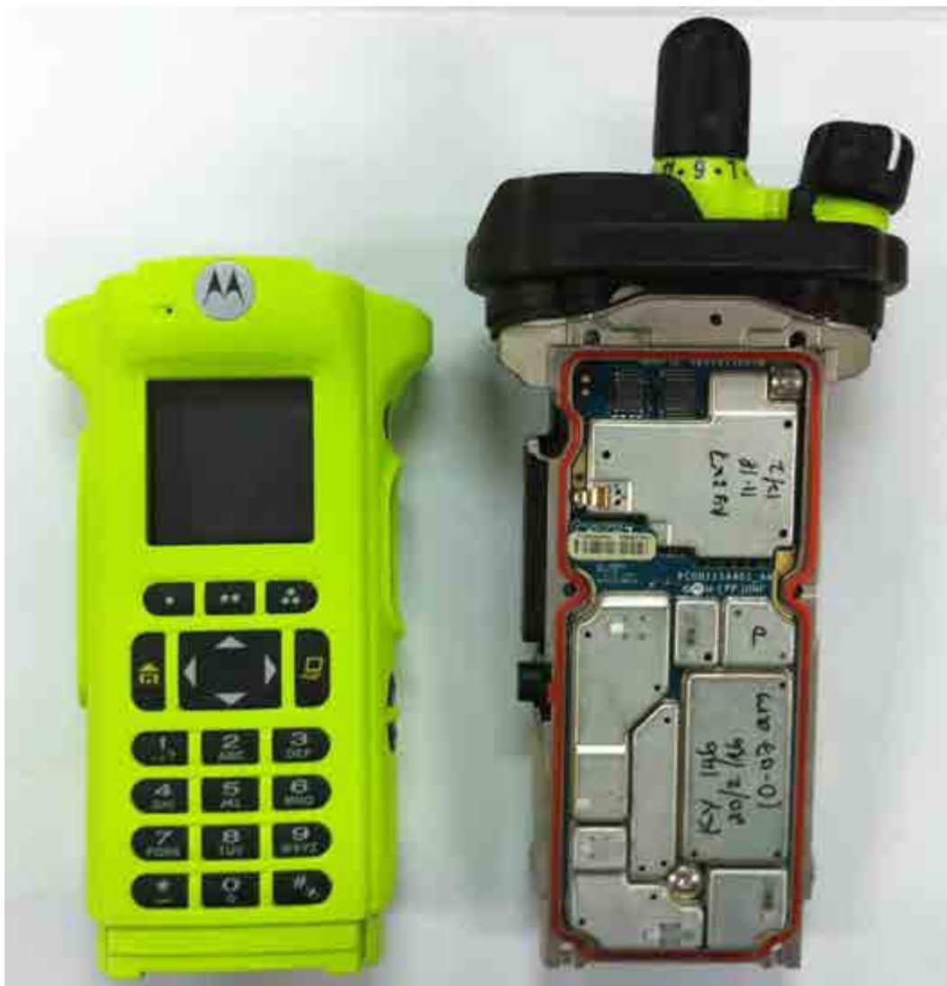
RF and Vocon boards with chassis and housing of APX6000XE Model 3.5 (Front side)
