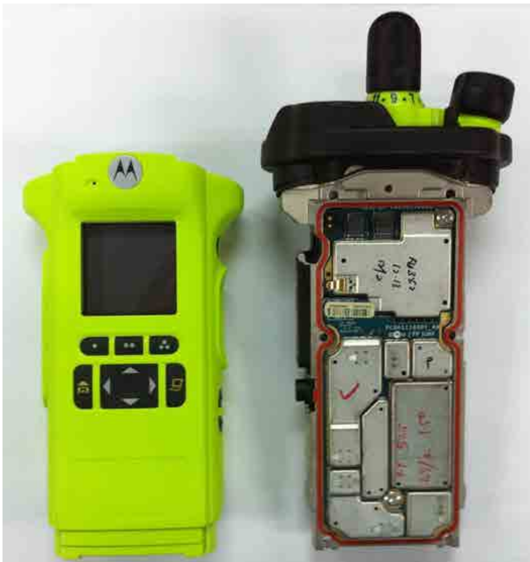
RF and Vocon boards with chassis and housing of APX6000XE Model 2.5 (Front side)
