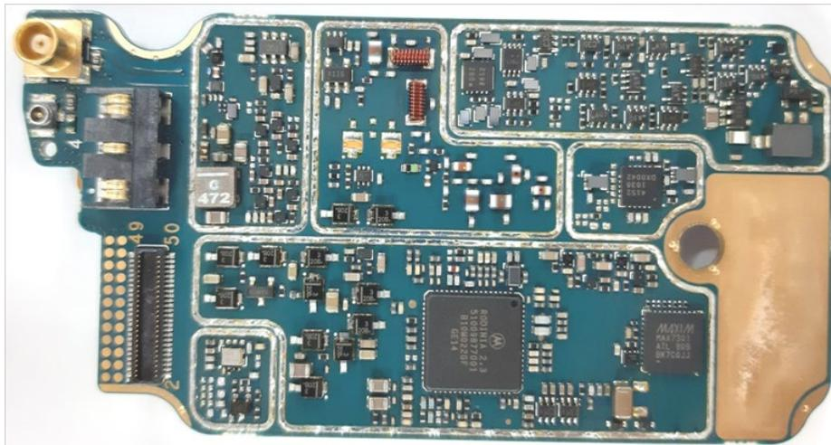
RF board without Shields (Bottom)
