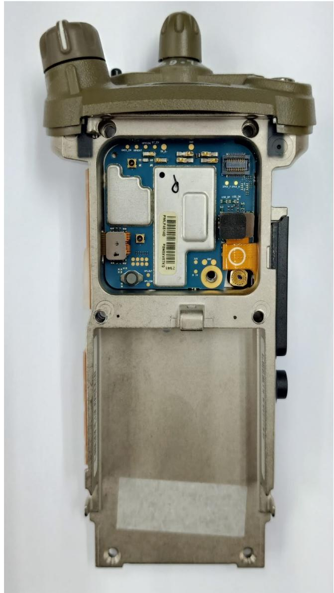
Expansion board with chassis and housing of Model 1.5 (Back side)
