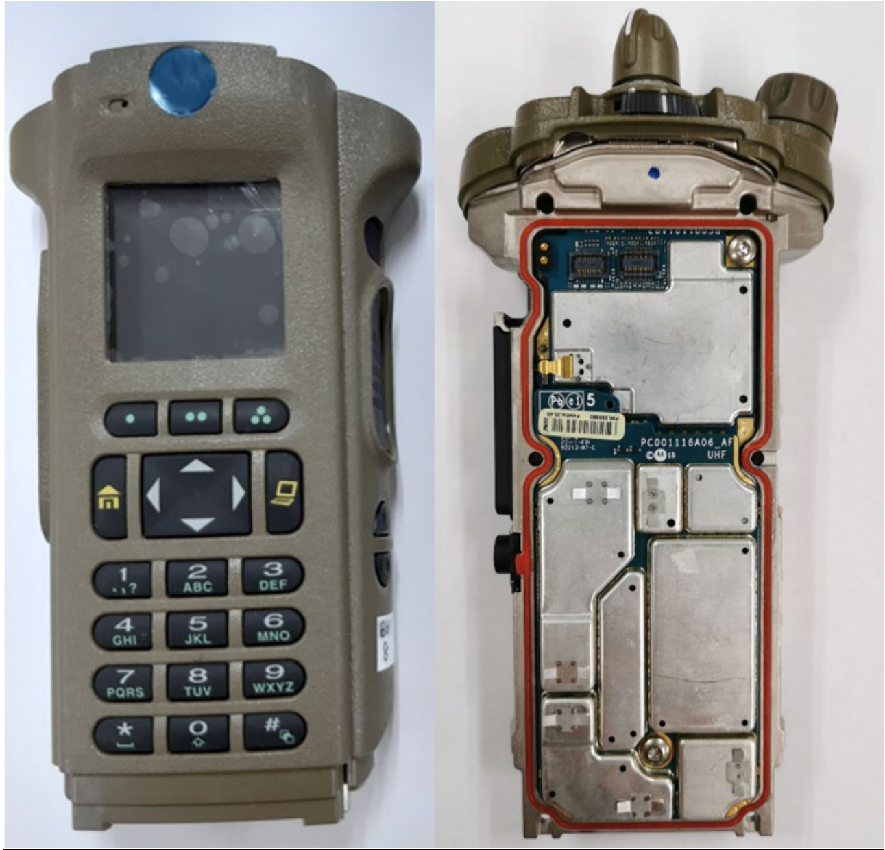
RF and Vocon boards with chassis and housing of SRX2200 Model 3.5 (Front side)
