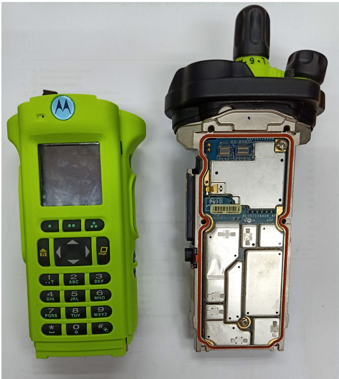
RF and Vocon boards with chassis and housing of APX6000XE Model 3.5 (Front side)
