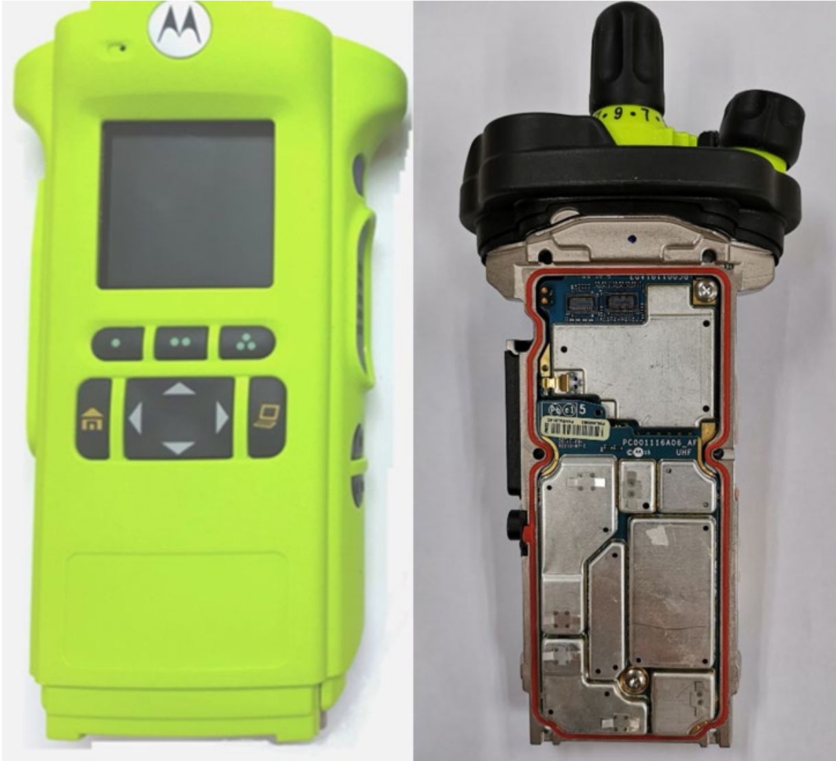
RF and Vocon boards with chassis and housing of APX6000XE Model 2.5 (Front side)
