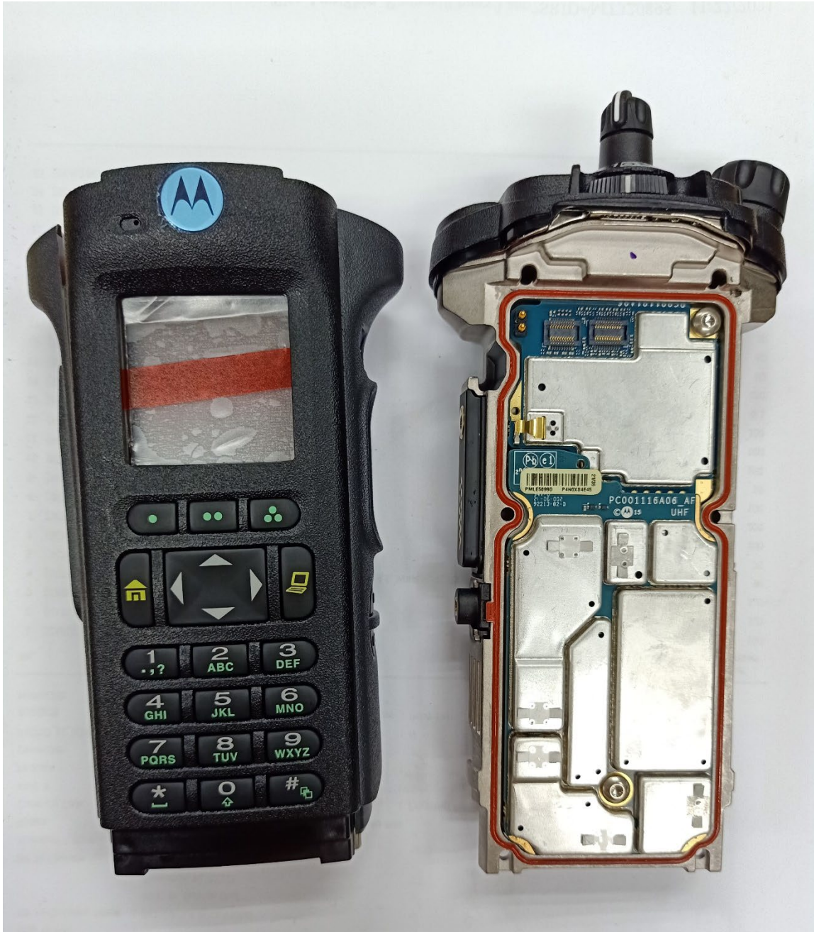
RF and Vocon boards with chassis and housing of APX6000/APX6000Li/APX5000 Model 3.5 (Front side)
