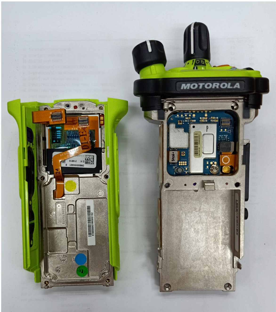
Expansion board with chassis and housing of APX6000XE Model 3.5 (Back side)
