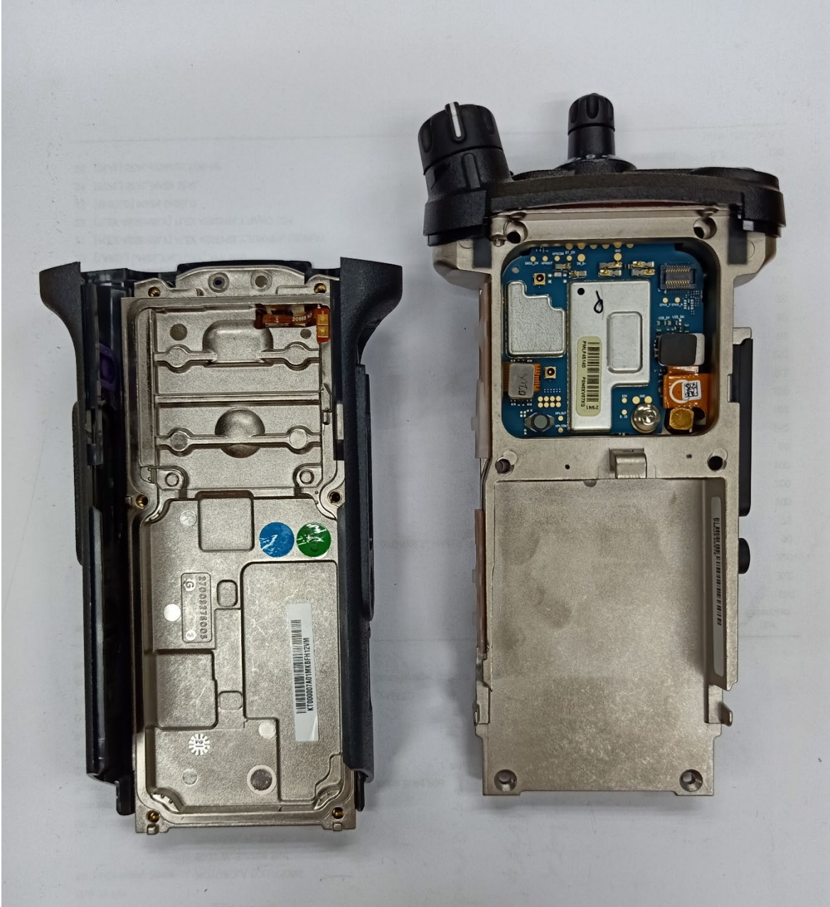
Expansion board with chassis and housing of APX6000/APX6000Li/APX5000 Model 1.5 (Back side)
