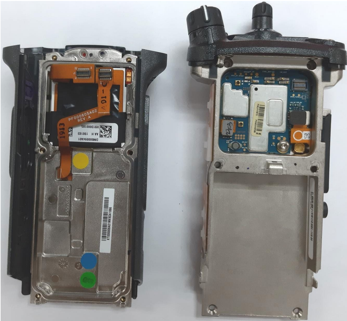
Expansion board with chassis and housing of APX6000/APX6000Li/APX5000 Model 2.5 (Back side)
