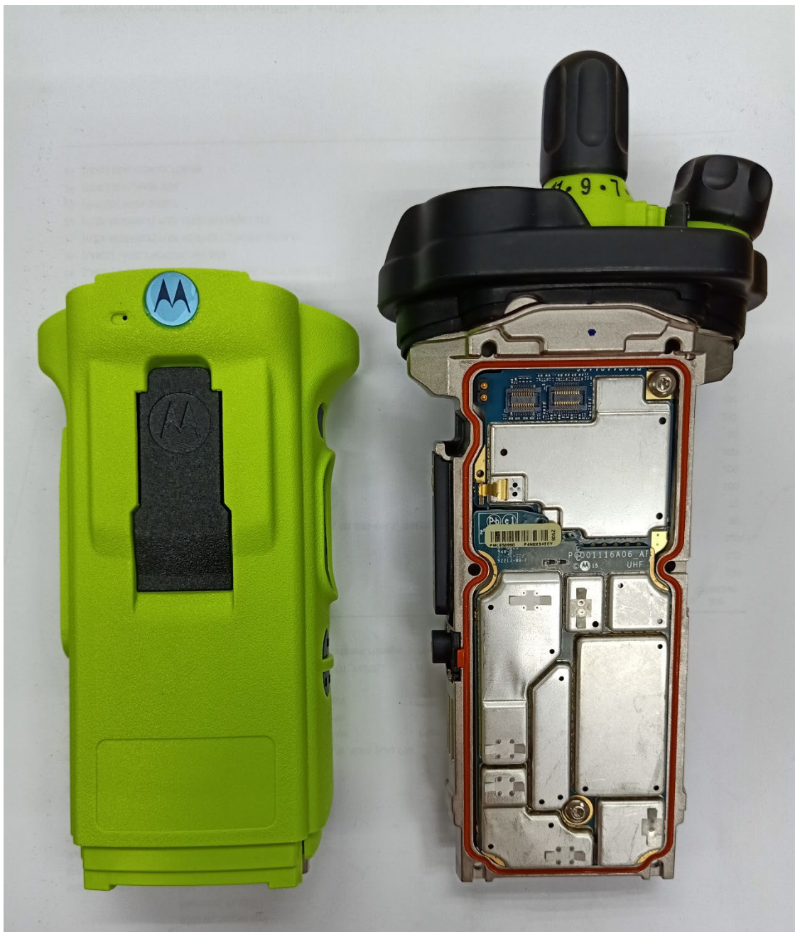
RF and Vocon boards with chassis and housing of APX6000XE Model 1.5 (Front side)
