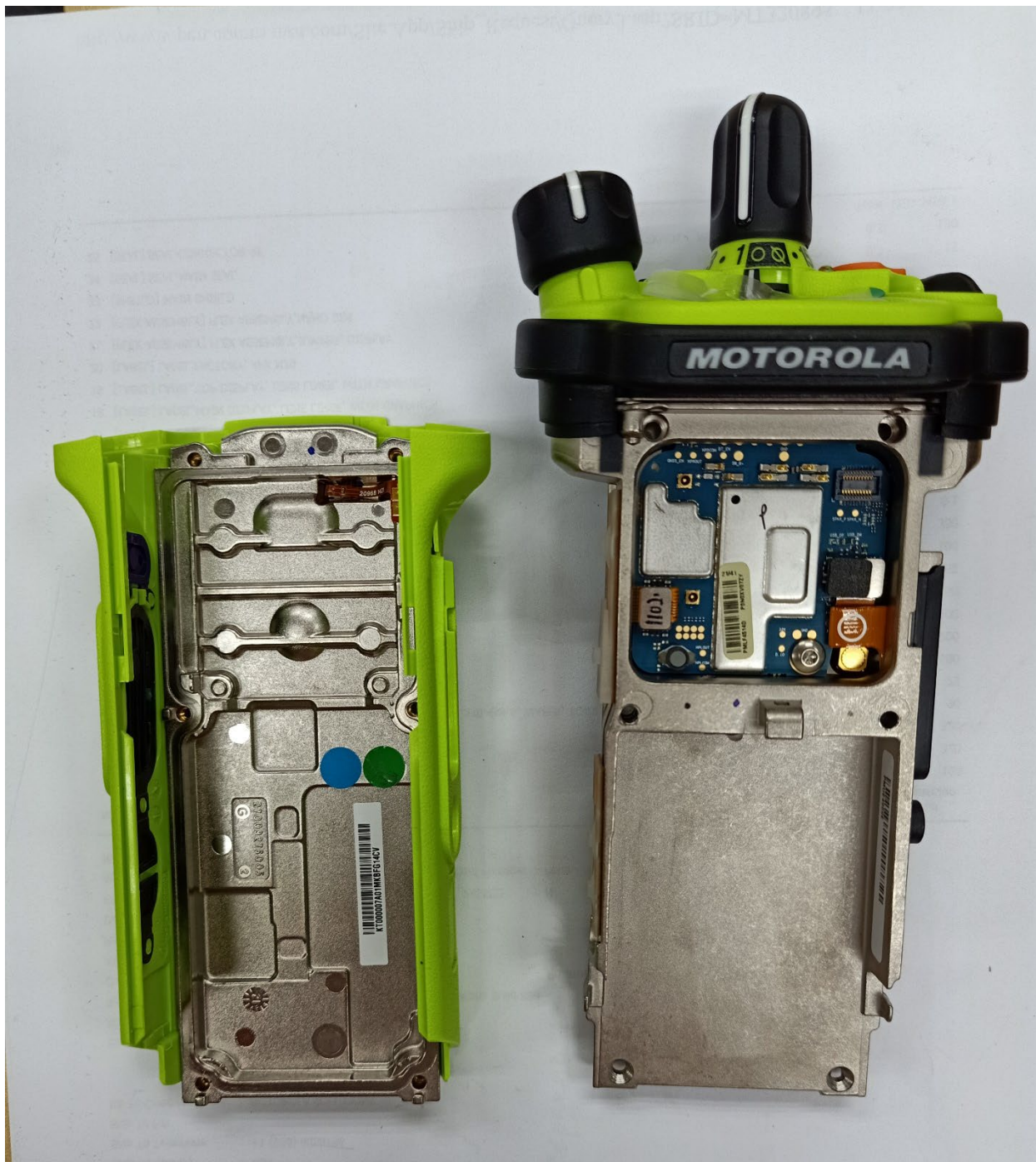
Expansion board with chassis and housing of APX6000XE Model 1.5 (Back side)
