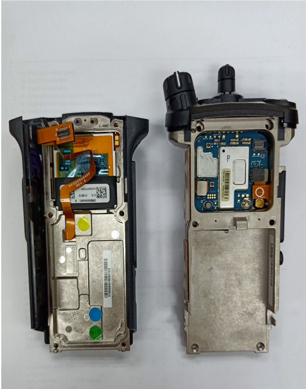
Expansion board with chassis and housing of APX6000/APX6000Li/APX5000 Model 3.5 (Back side)
