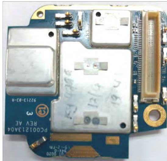
Expansion board with shields (Bottom) (APX6000/APX5000/APX6000XE/APX6000Li/SRX2200)
