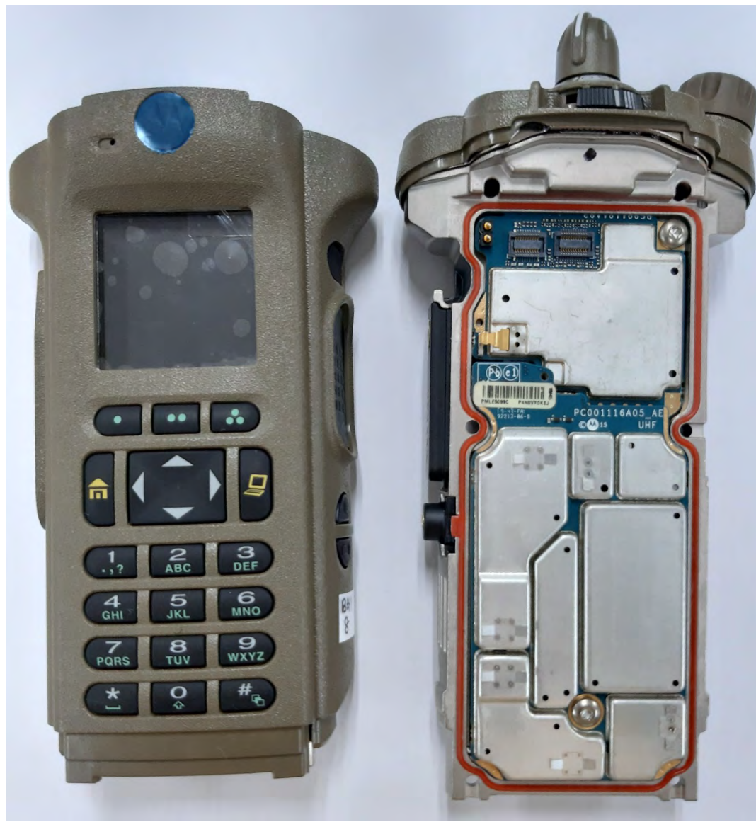
RF and Vocon boards with chassis and housing of SRX2200 Model 3.5 (Front side)
