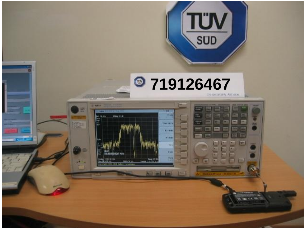
Peak Power Spectral Density Test Setup
