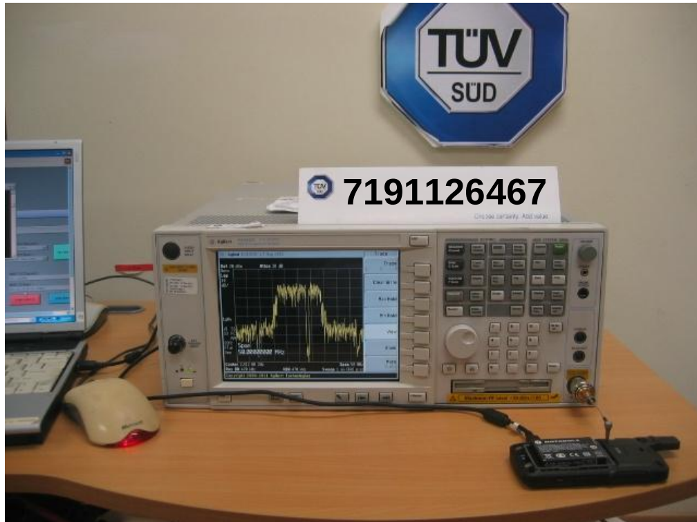
Band Edge Compliance (Conducted) Test Setup
