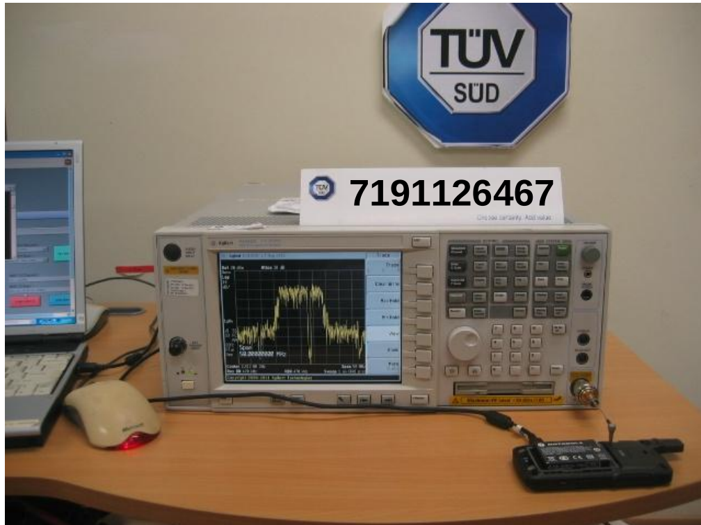
Spectrum Bandwidth (6dB Bandwidth Measurement) Test Setup
