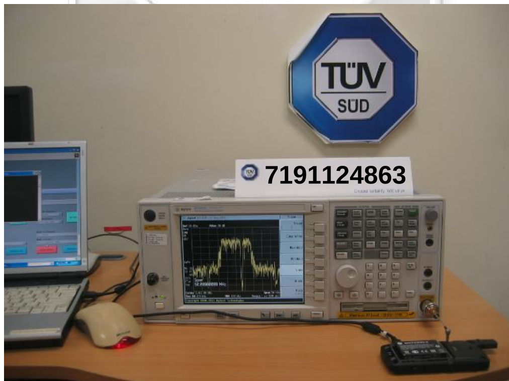
Average Frequency Dwell Time Test Setup
