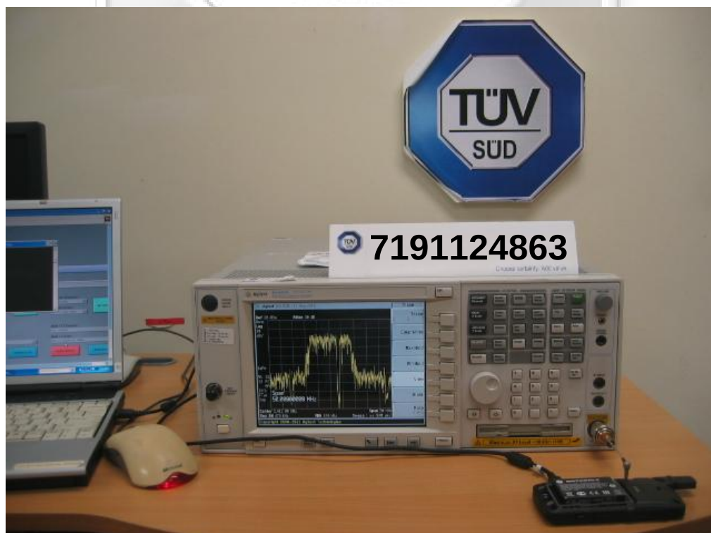
RF Conducted Spurious Emissions Test Setup
