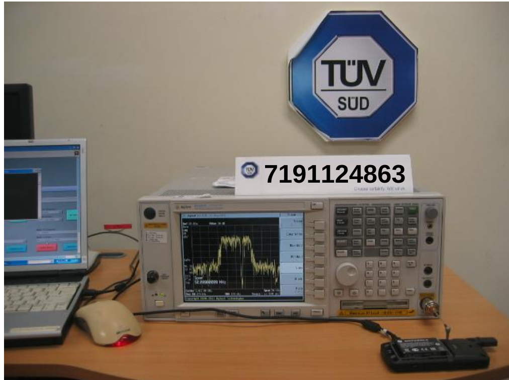
Band Edge Compliance (Conducted) Test Setup
