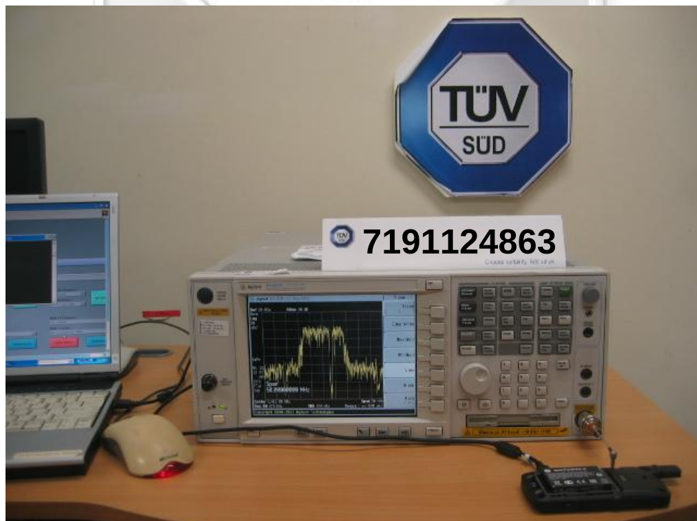
Spectrum Bandwidth (20dB Bandwidth Measurement) Test Setup
