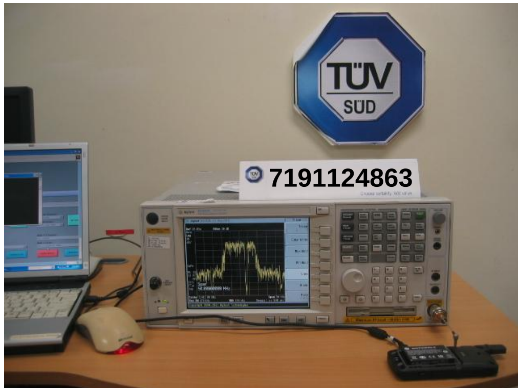
Peak Power Spectral Density Test Setup
