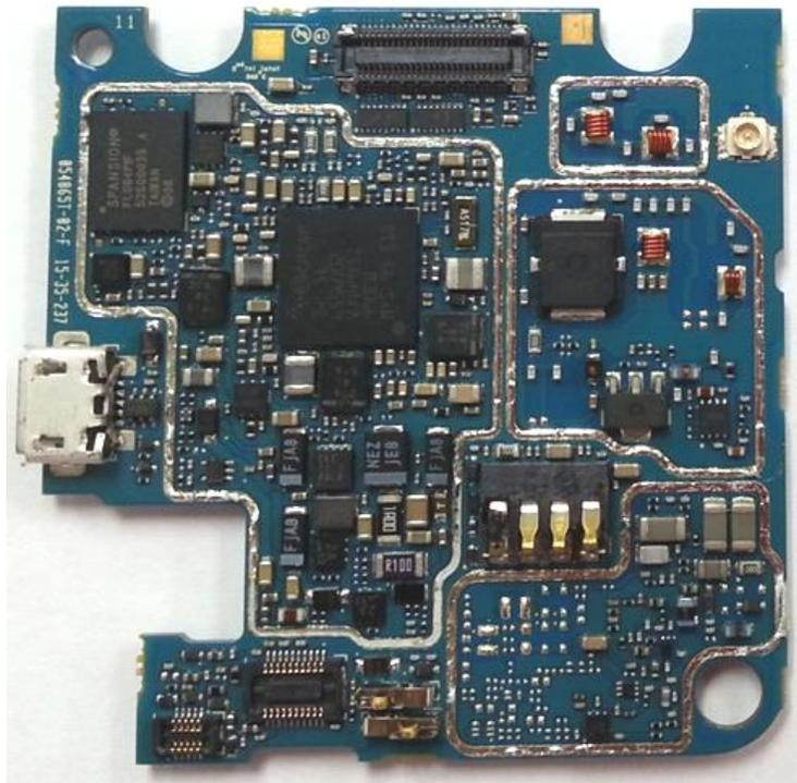
RF board **without** Shields (Bottom)
