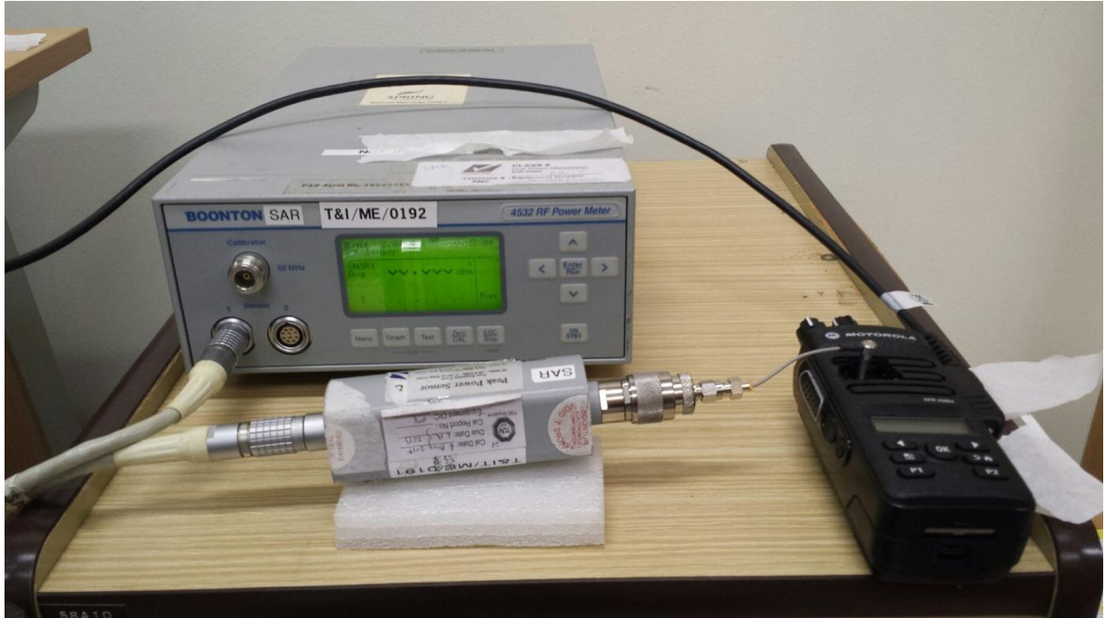
Maximum Peak Power Test Setup
