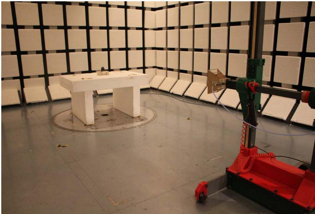
**1.3. Radiated Emission test setup photo for LMR (ISED – ANSI C63.26:2015)**
