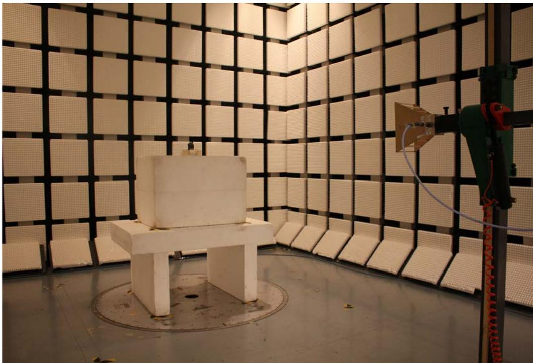
**1.4. Radiated Emission test setup photo for BT/BT LE/WLAN 2.4GHz (ANSI C63.10: 2013)**
