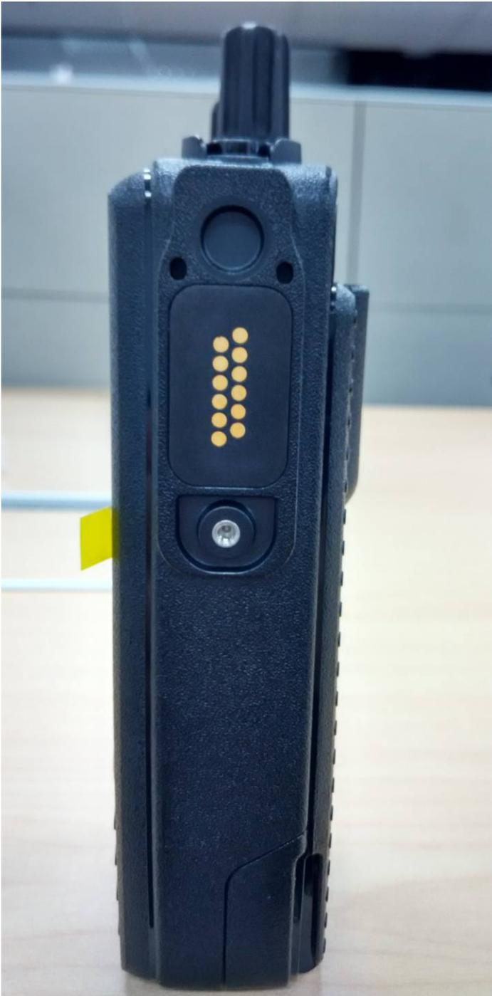
**Side View for Keypad and Plain (SMA) Model (Left) – New model**
