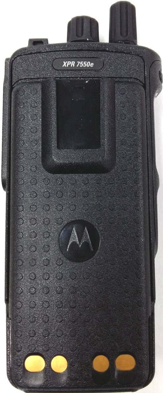
Back View with Battery For Keypad and Plain Model – Current and new model
