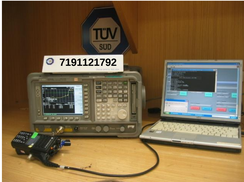
Number of Hopping Frequencies Test Setup
