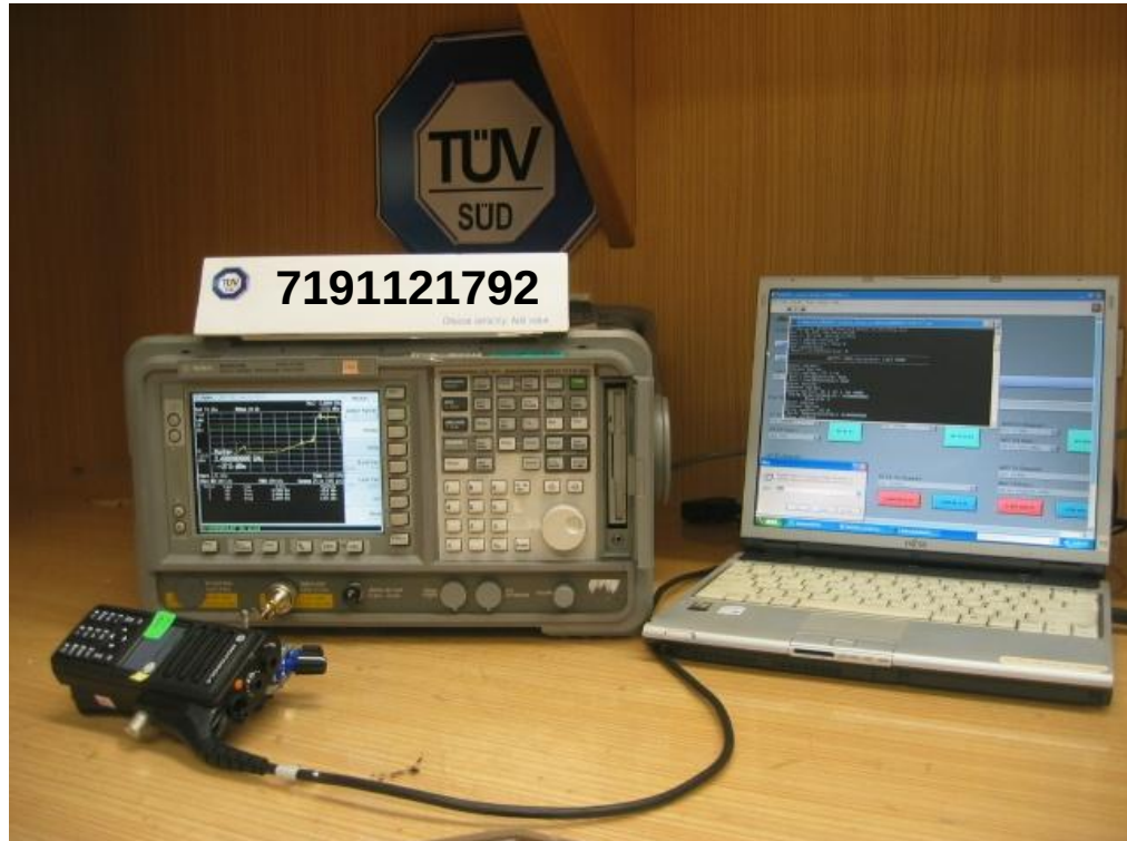
Band Edge Compliance (Conducted) Test Setup
