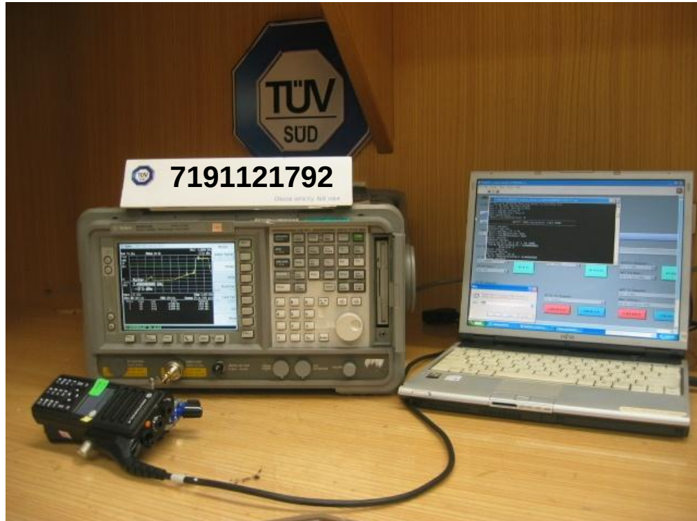
Carrier Frequency Separation Test Setup
