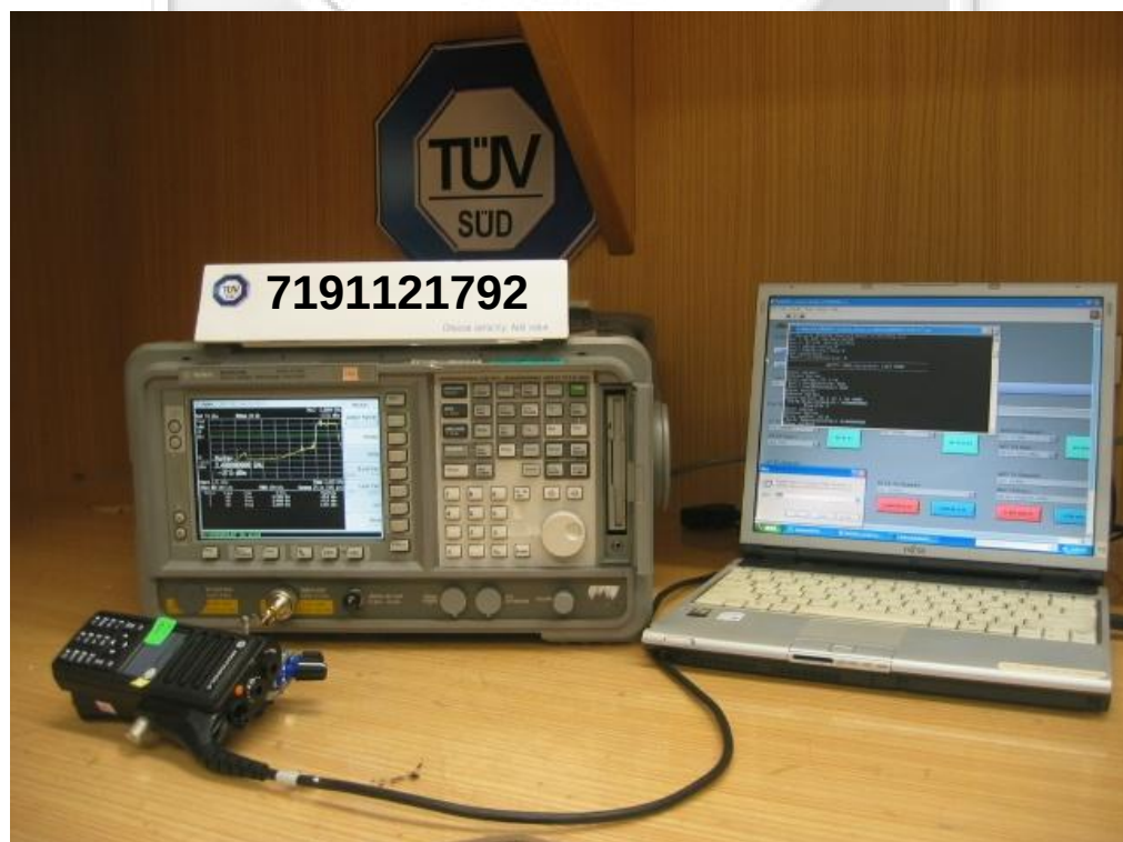
RF Conducted Spurious Emissions Test Setup
