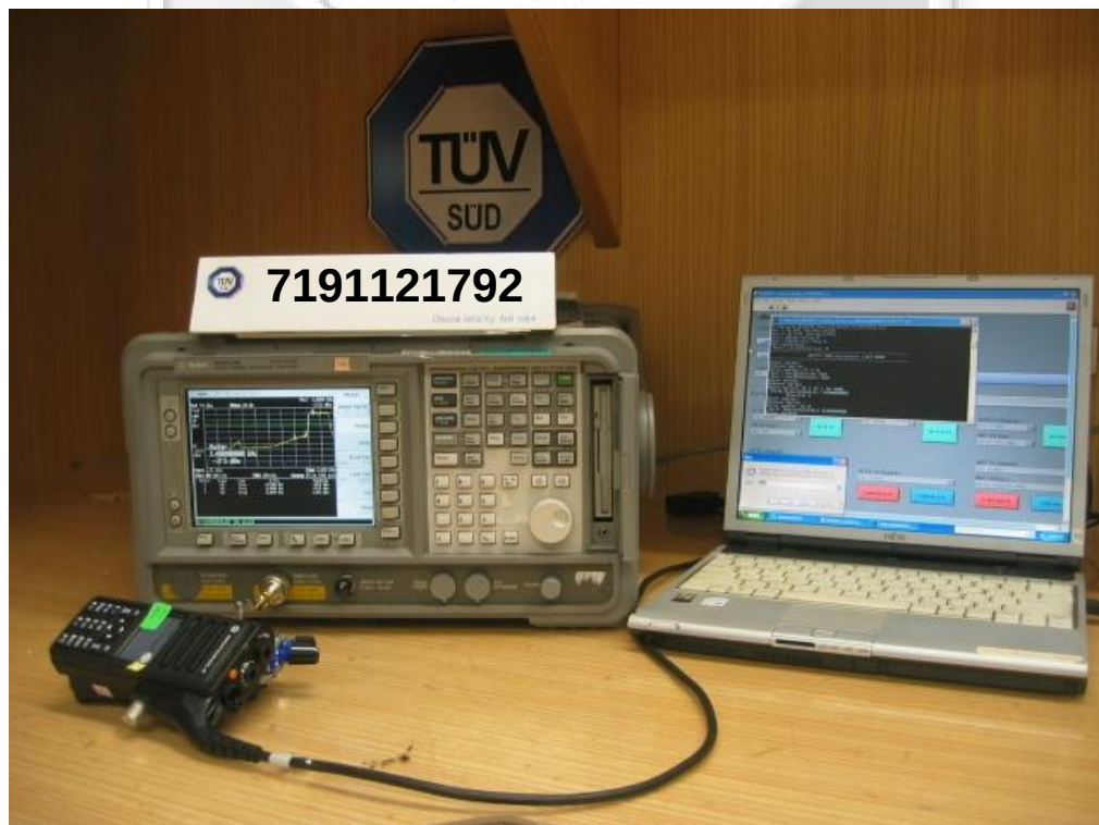
Average Frequency Dwell Time Test Setup
