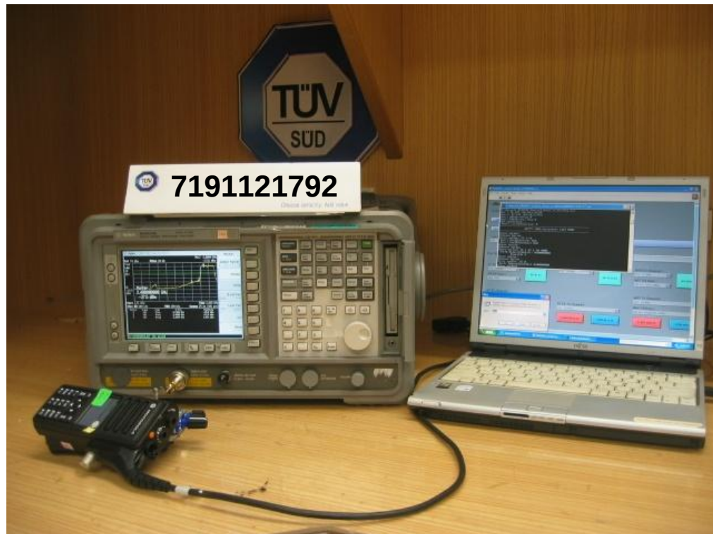
Peak Power Spectral Density Test Setup
