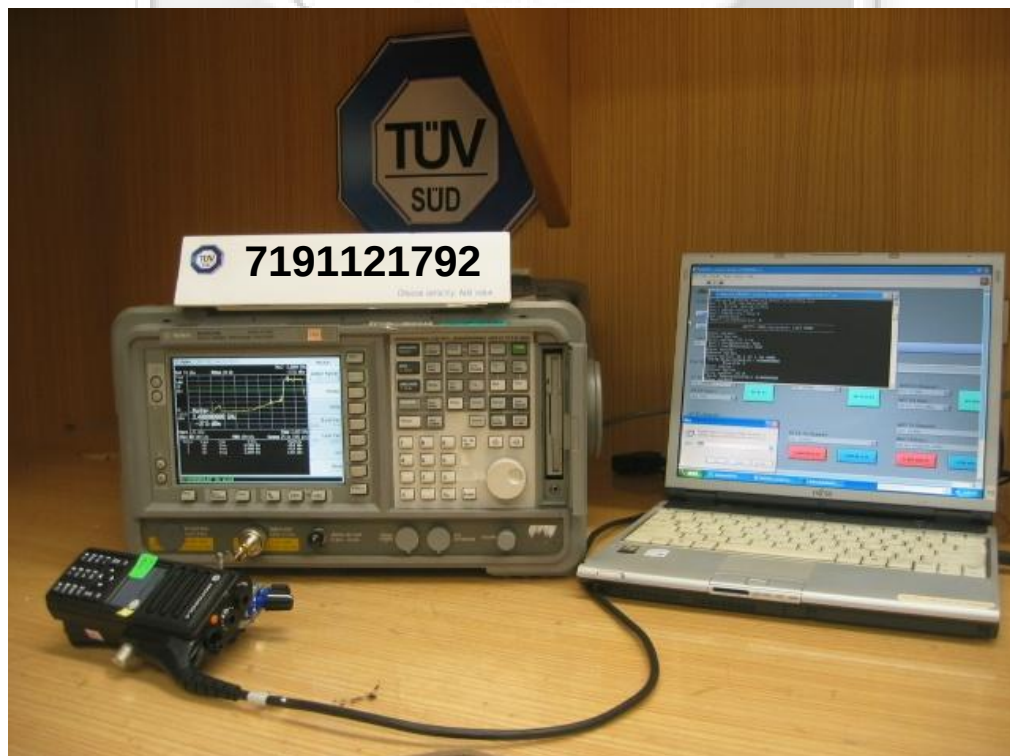
Spectrum Bandwidth (20dB Bandwidth Measurement) Test Setup
