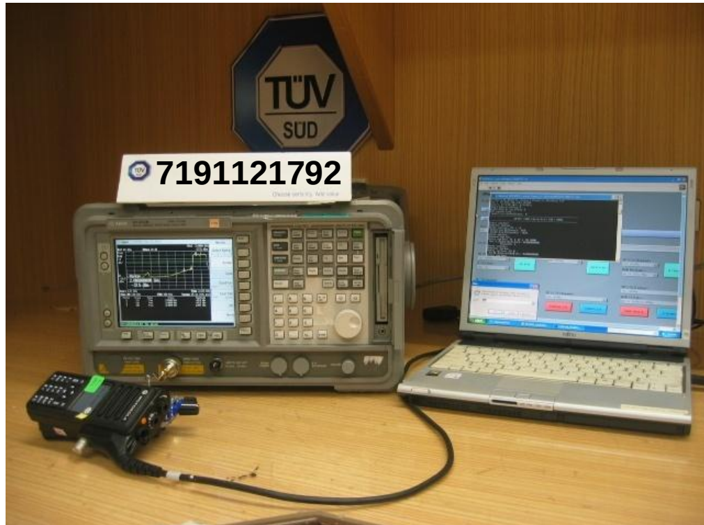
Spectrum Bandwidth (6dB Bandwidth Measurement) Test Setup
