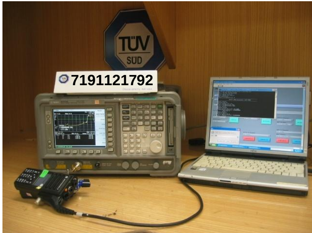
Band Edge Compliance (Conducted) Test Setup
