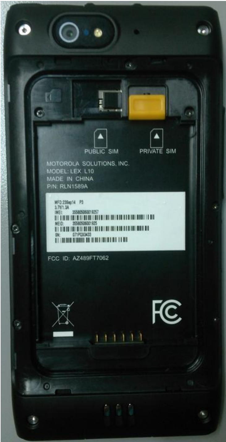
Figure 3-7. Detail of Regulatory Markings
