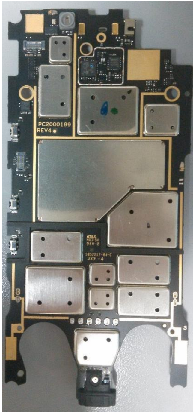
Photograph 9-1: Top side of main board, shields in place
