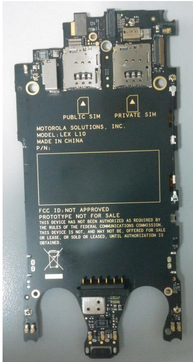
Photograph 9-2: Bottom side of main board, shields in place
