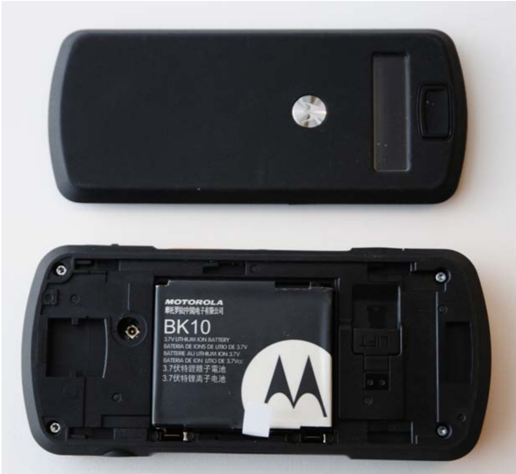
Photograph 3 – EWP2200 Rear View Battery Cover Removed
