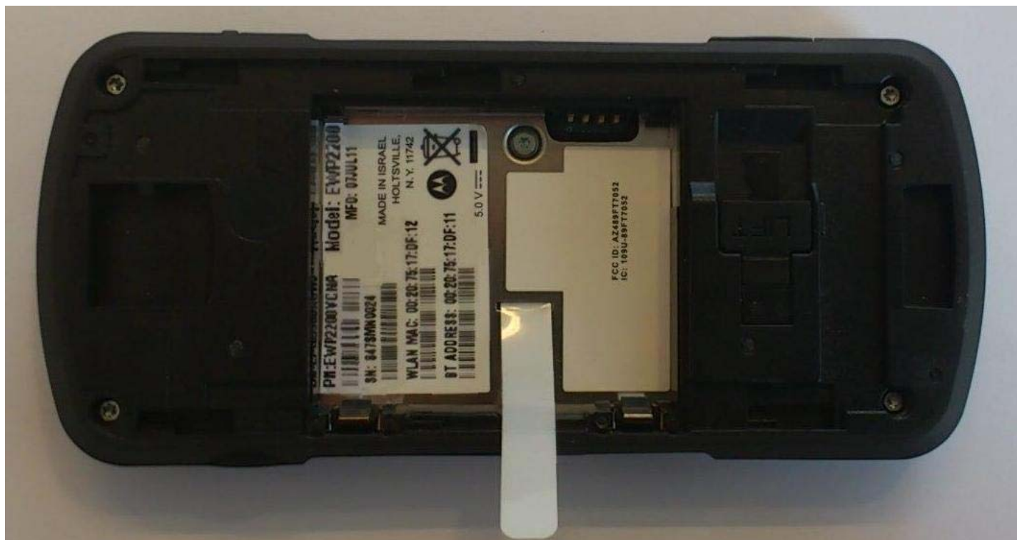
Photograph 4 – EWP2200 Rear View Battery Removed
