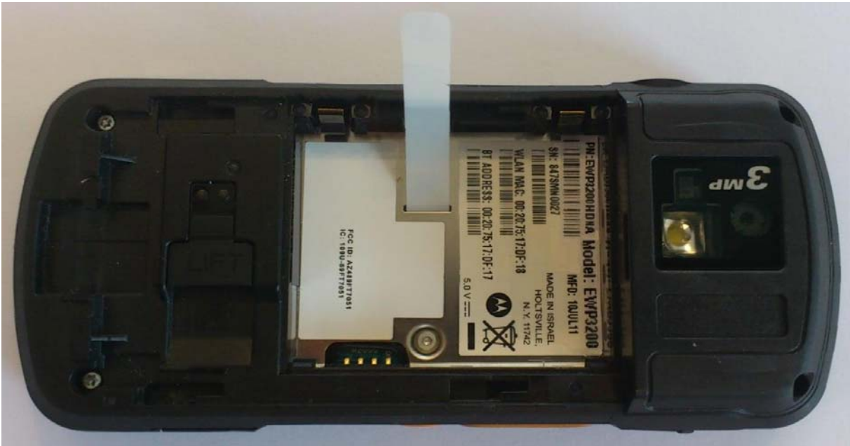
Photograph 3 – EWP3200 Rear View Battery Cover Removed
