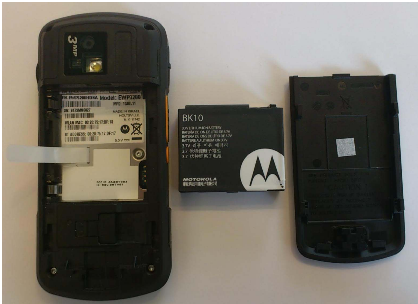
Photograph 5 – EWP3200 Assembly of Battery and Battery Cover
