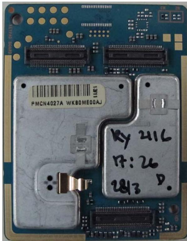
Keypad board with Shields (Bottom)
