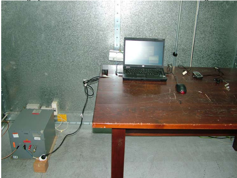
Photograph 3: Power Line Emissions measurement, PC configuration
