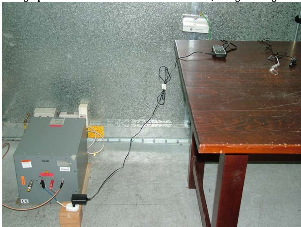
Photograph 2: Power Line Emissions measurement, charger configuration
