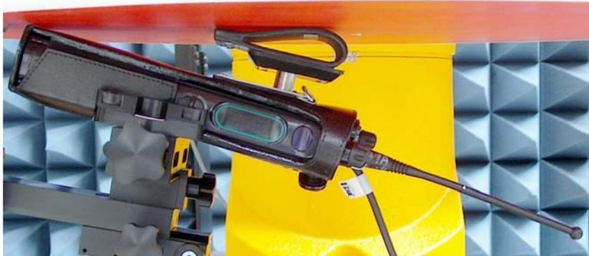
DUT with carry accessory PMLN5330A/PMLN5408A 2.75" swivel loop against the phantom. Audio accessory HMN4104A attached.
