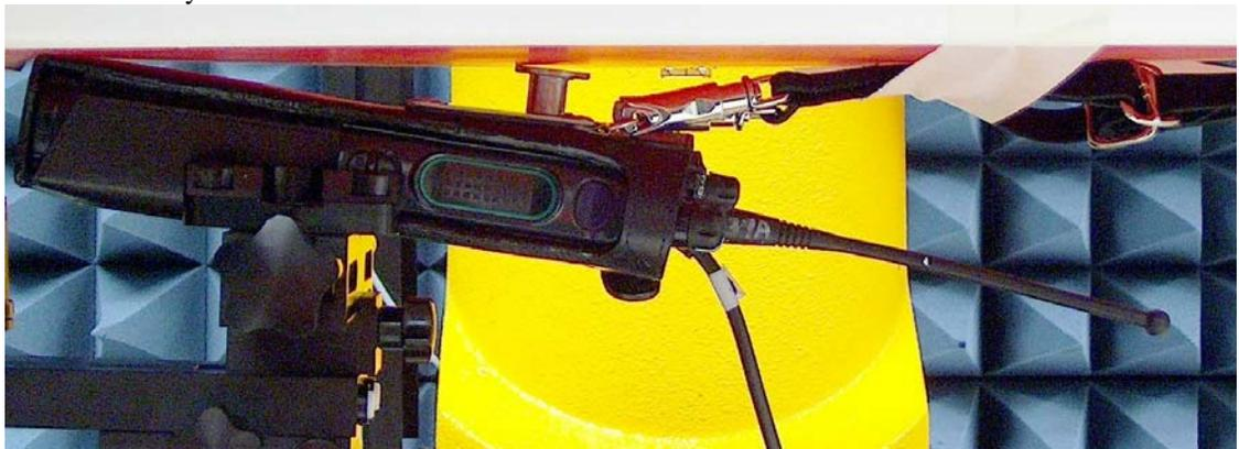
DUT with PTT side against the phantom with carry accessory PMLN5330A and NTN5243A. Audio accessory HMN4104A attached.
