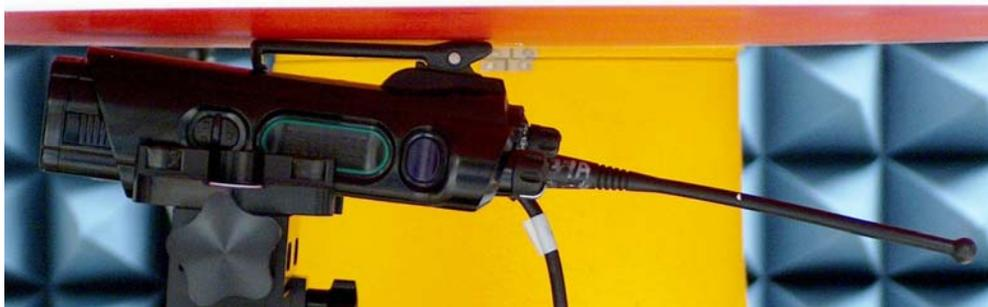
DUT with accessory side against the phantom with carry accessory PMLN5322A and NTN5243A. Audio accessory HMN4104A attached.
