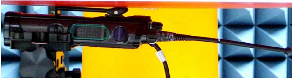
DUT with carry accessory PMLN5322A against the phantom. Audio accessory HMN4104A attached.
