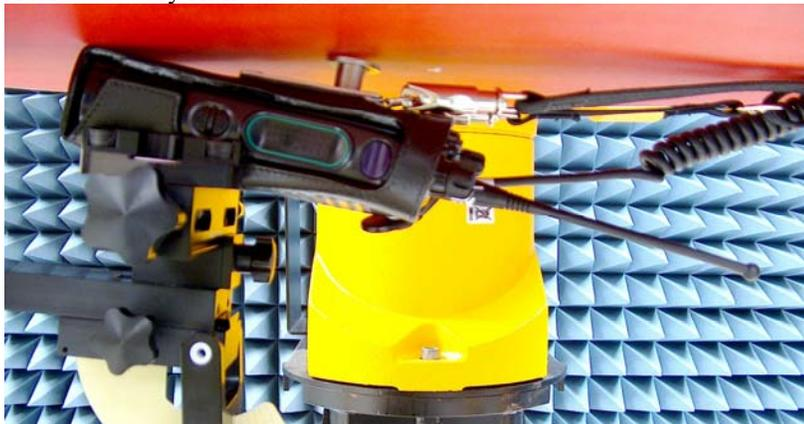
DUT with PTT side against the phantom with carry accessory PMLN5324A and NTN5243A. Audio accessory HMN4104A attached.
