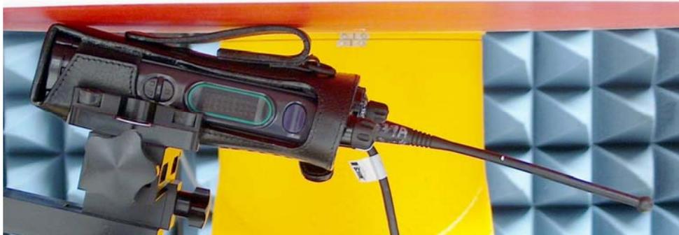
DUT with carry accessory PMLN5324A/PMLN5407A 2.5" swivel loop against the phantom. Audio accessory HMN4104A attached.
