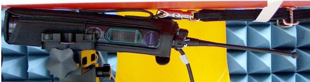
DUT with PTT side against the phantom with carry accessory PMLN5328A and NTN5243A. Audio accessory HMN4104A attached.
