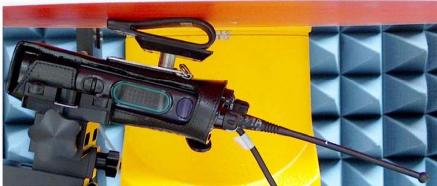
DUT with carry accessory PMLN5324A/PMLN5408A 2.75" swivel loop against the phantom. Audio accessory HMN4104A attached.
