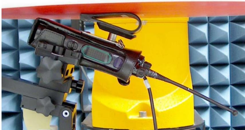
DUT with carry accessory PMLN5324A/PMLN5409A 3.0" swivel loop against the phantom. Audio accessory HMN4104A attached.
