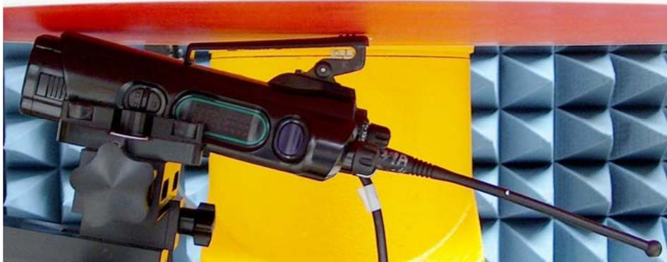
DUT with carry accessory PMLN5331A and belt clip NTN8266B against the phantom.
