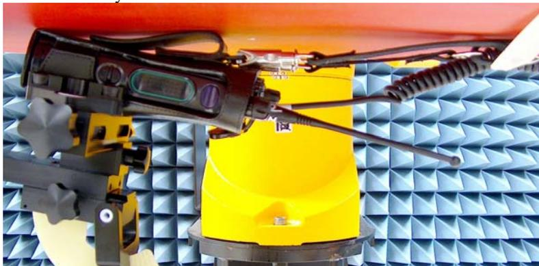
DUT with PTT side against the phantom with carry accessory PMLN5323A and NTN5243A. Audio accessory HMN4104A attached.
