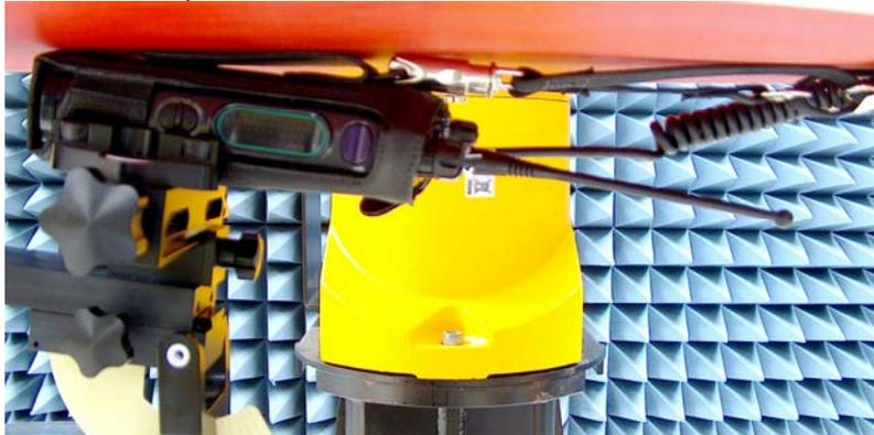
DUT with PTT side against the phantom with carry accessory PMLN5322A and NTN5243A. Audio accessory HMN4104A attached.
