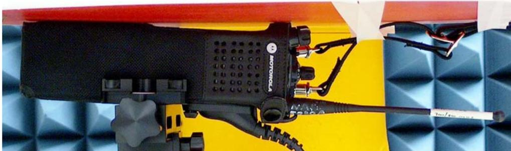
DUT with accessory side against the phantom with carry accessory PMLN5329A and NTN5243A. Audio accessory HMN4104A attached.
