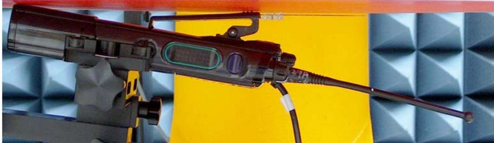
DUT with belt clip NTN8266B against the phantom. Audio accessory HMN4104A attached.
