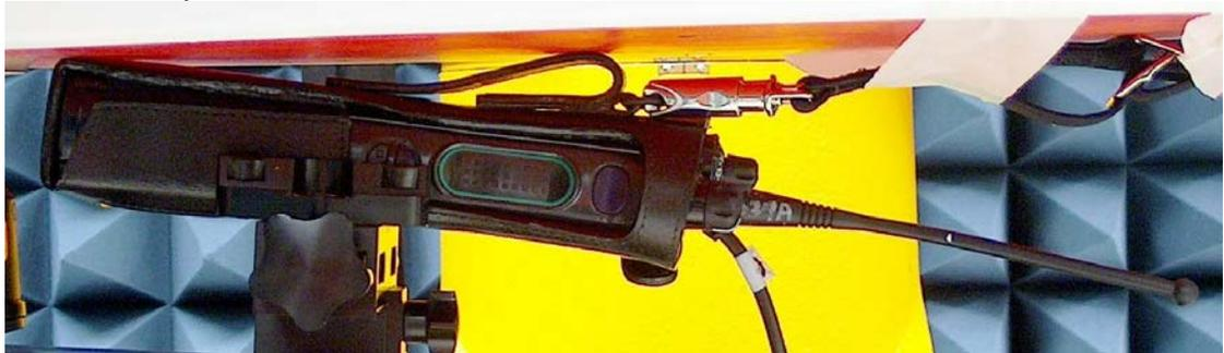
DUT with PTT side against the phantom with carry accessory PMLN5329A and NTN5243A. Audio accessory HMN4104A attached.
