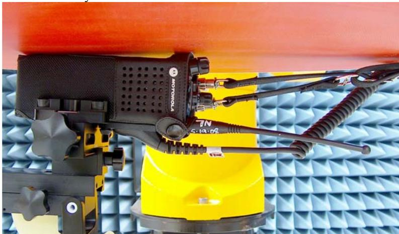
DUT with accessory side against the phantom with carry accessory PMLN5323A and NTN5243A. Audio accessory HMN4104A attached.
