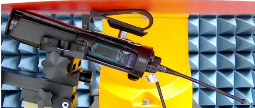
DUT with carry accessory PMLN5330A/PMLN5409A 3.0" swivel loop against the phantom. Audio accessory HMN4104A attached.
