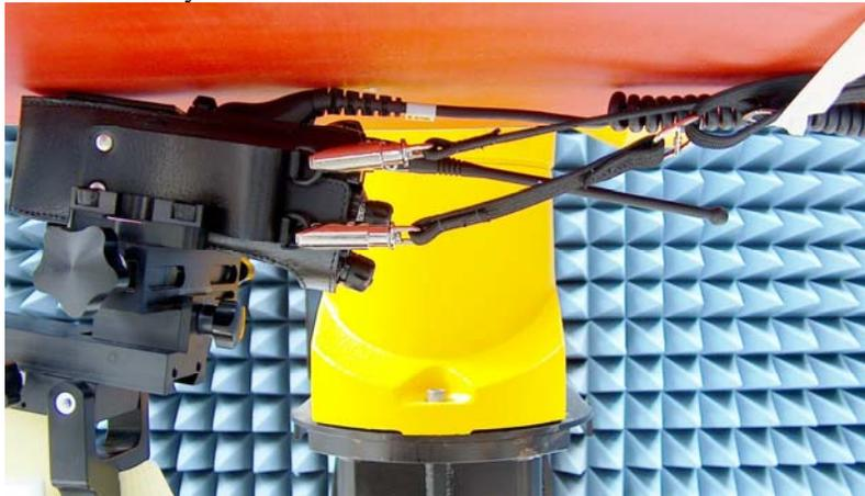
DUT with back side against the phantom with carry accessory PMLN5323A and NTN5243A. Audio accessory HMN4104A attached.
