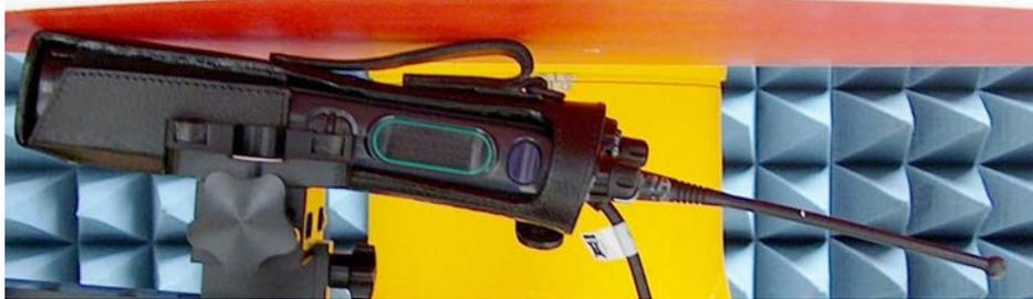
DUT with carry accessory PMLN5331A and belt clip HLN6875A against the phantom.
