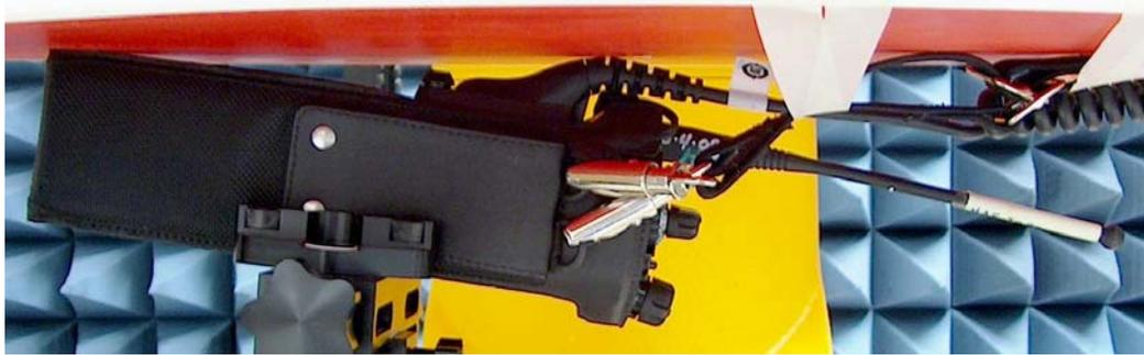
DUT with back side against the phantom with carry accessory PMLN5328A and NTN5243A. Audio accessory HMN4104A attached.
