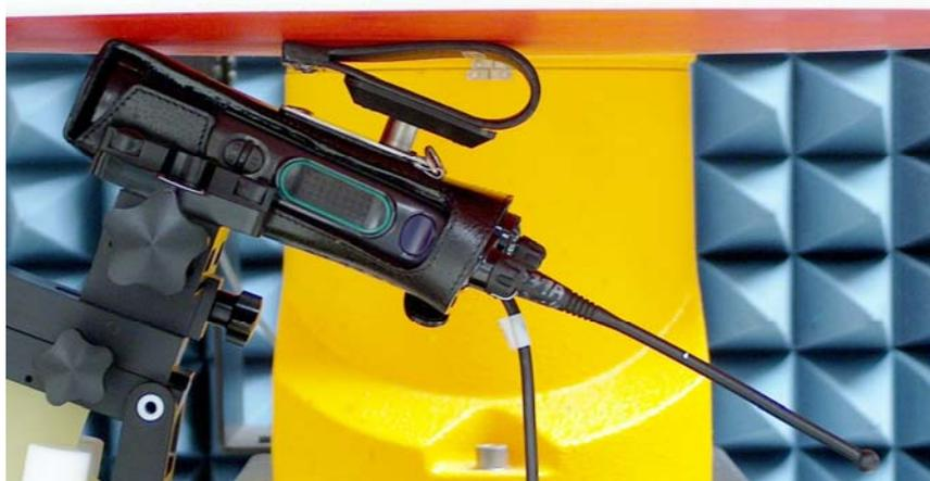
DUT with carry accessory PMLN5330A/PMLN5407A 2.5" swivel loop against the phantom. Audio accessory HMN4104A attached.
