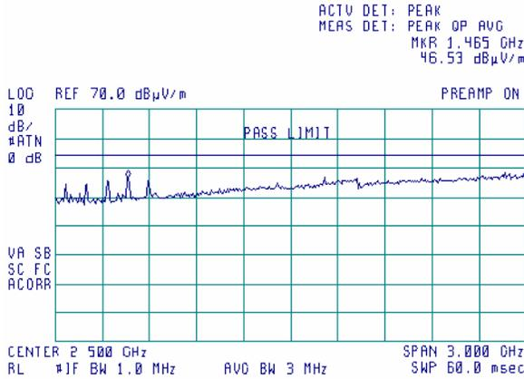
**Plot 9.2.4 Radiated emission measurements in 1000 - 4000 MHz range, horizontal antenna polarization**
