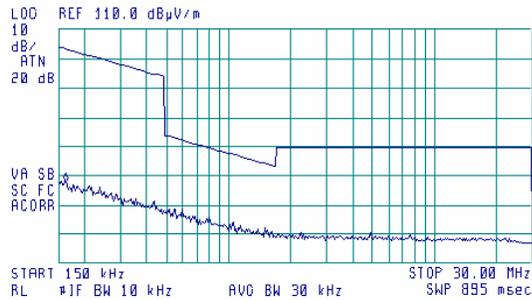
**Plot 7.3.14 Radiated emission measurements from 0.15 to 30 MHz at the mid carrier frequency**
