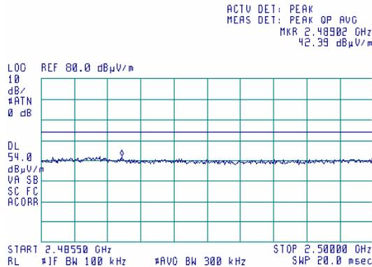
\* - 2483.5 to 2485.5 MHz band was investigated in band edge emission as provided in plot 7.3.89 to plot 7.3.98.
