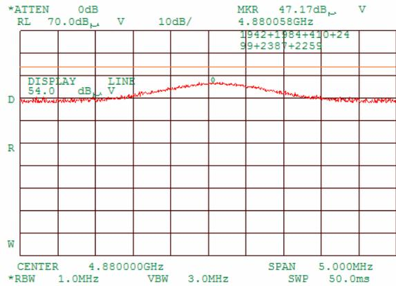
Plot 7.3.60 Radiated emission measurements at the second harmonic of mid carrier frequency
