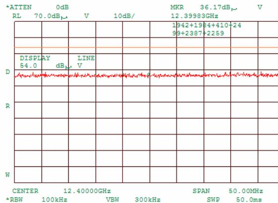
**Plot 7.3.88 Radiated emission measurements at the fifth harmonic of high carrier frequency**
