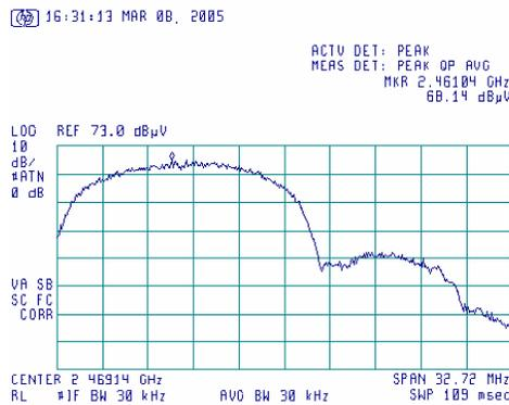
**Plot 7.3.98 Radiated emission measurements at band edge**
