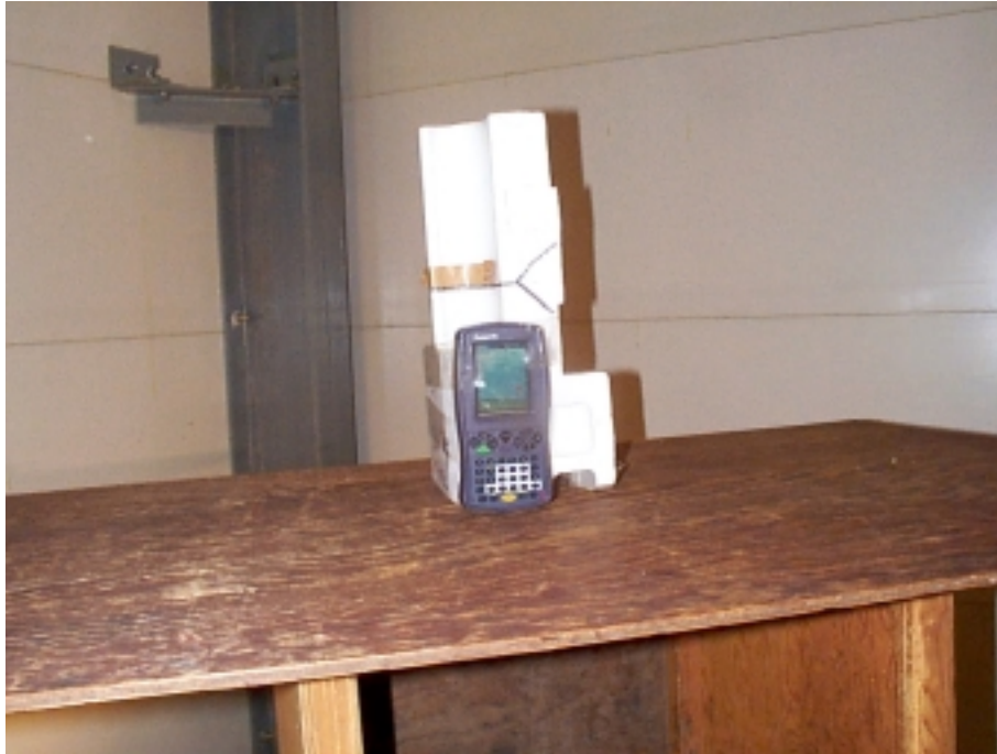
View of EPad Terminal On It's Back as it was when measuring the Part 15.109
