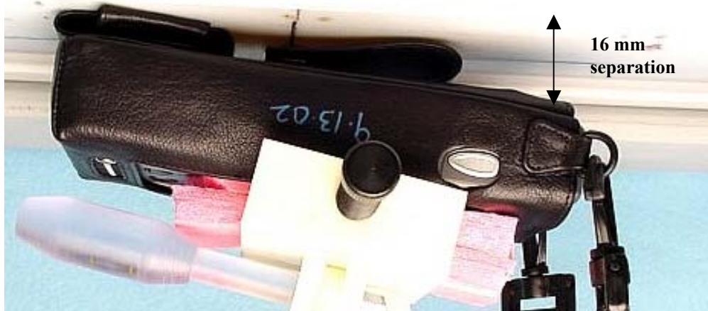
Figure 8. Assessment @ the Abdomen; Backside of DUT towards the phantom w/ battery model FNN5105A and carry case model FHN6396A
