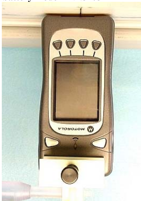
Figure 3. Assessment @ the Abdomen; bottom side of DUT against the phantom w/ battery model FNN5105A
