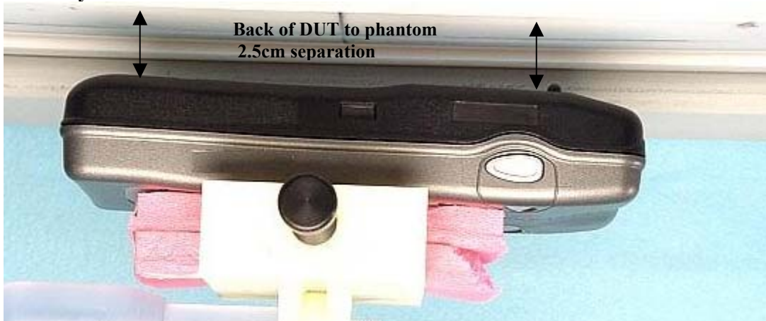
Figure 10. Assessment @ abdomen; Back of DUT 2.5cm separation distance w/ battery model FNN5105A
