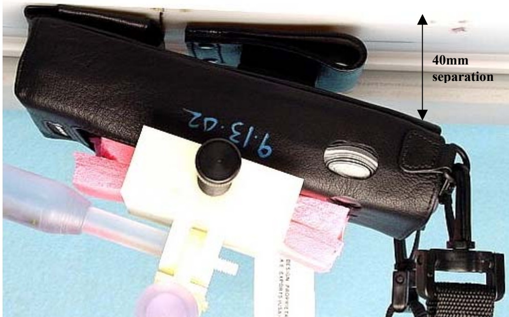
Figure 6. Assessment @ the Abdomen; Backside of DUT towards the phantom w/ battery model FNN5105A and carry case model FHN6395A
