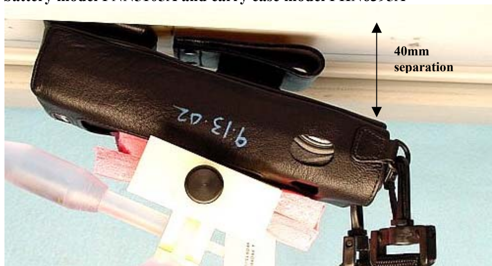
Figure 7. Assessment @ the Abdomen; Display side of DUT towards the phantom w/ battery model FNN5105A and carry case model FHN6395A
