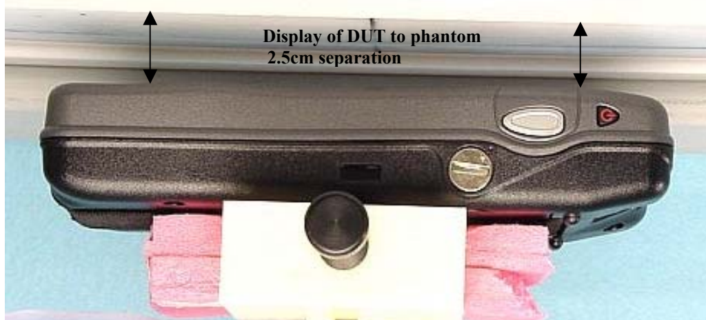
Figure 11. Assessment @ the Abdomen; Display of DUT 2.5cm separation distance w/ battery model FNN5105A
