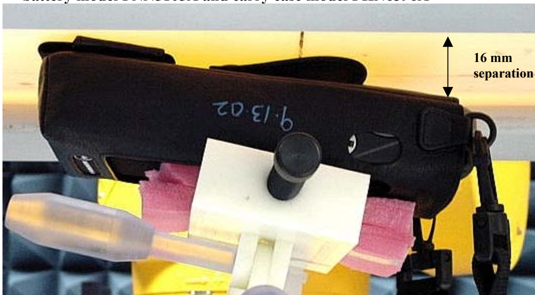
Figure 9. Assessment @ the Abdomen; Display side of DUT towards the phantom w/ battery model FNN5105A and carry case model FHN6396A
