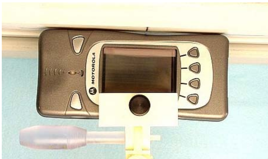
Figure 4. Assessment @ the Abdomen; Right side of DUT against the phantom w/ battery model FNN5105A
