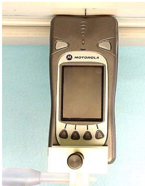
Figure 2. Assessment @ the Abdomen; Top side of DUT against the phantom w/ battery model FNN5105A
