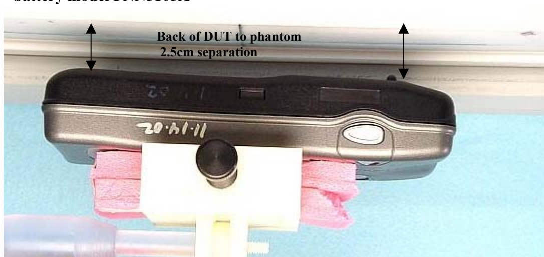
Figure 10. Assessment @ abdomen; Back of DUT 2.5cm separation distance w/ battery model FNN5105A
