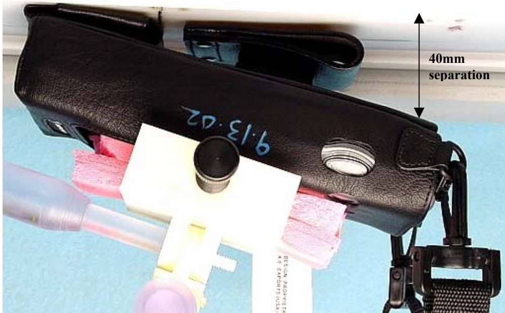
Figure 6. Assessment @ the Abdomen; Backside of DUT towards the phantom w/ battery model FNN5105A and carry case model FHN6395A
