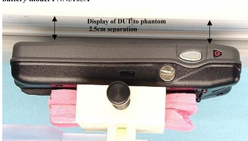
Figure 11. Assessment @ the Abdomen; Display of DUT 2.5cm separation distance w/ battery model FNN5105A
