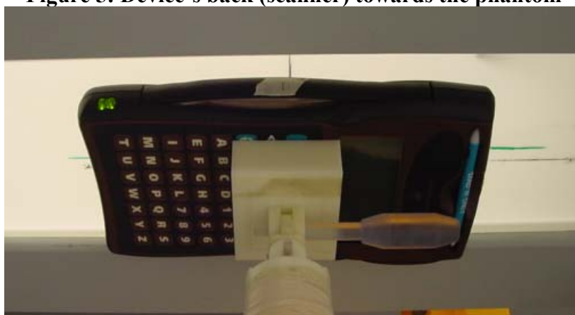
Figure 5: Device's back (scanner) towards the phantom
