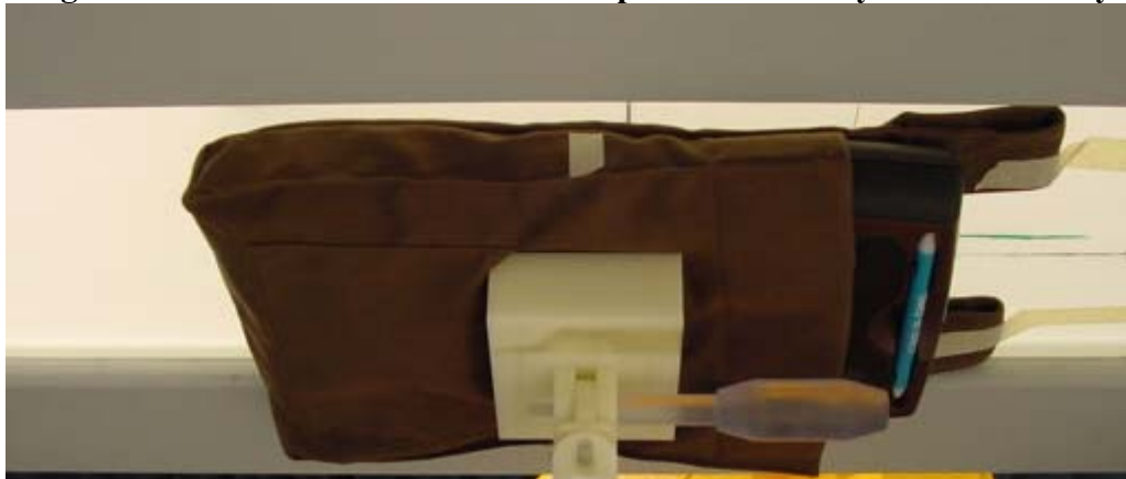
Figure 7: Device with scanner towards phantom in body worn accessory
