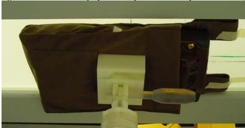
Figure 6: Device with display towards phantom in body worn accessory
