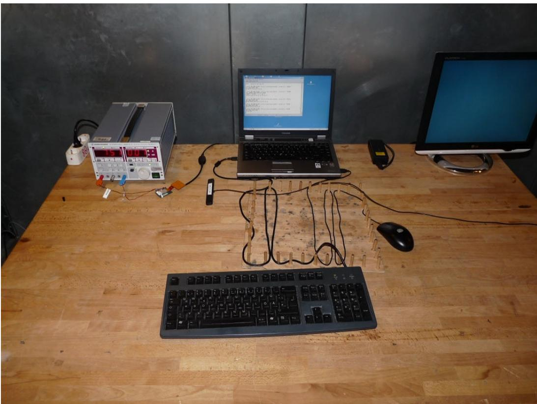
**Photo 4:** Test setup for Conducted emissions (AC power line)
