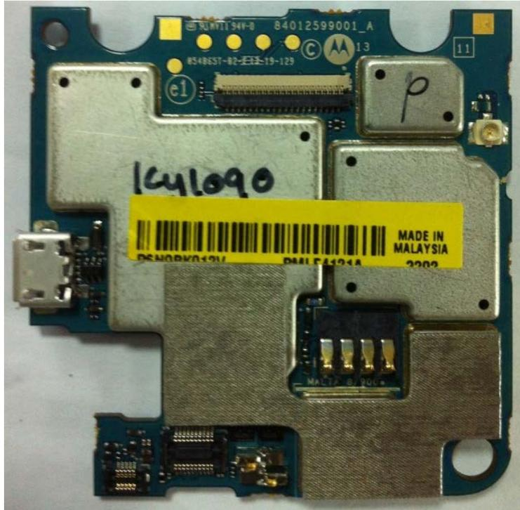
RF board **with** Shields (Bottom)
