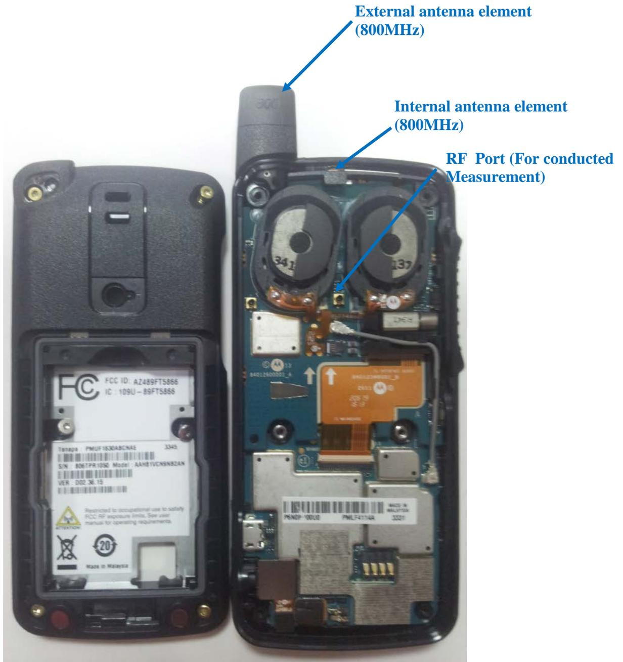
PCB board with housing (Back)
