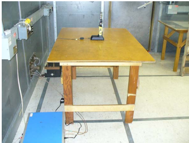
Figure 4.2.4-2: Conducted Emissions Test Setup – Side View
