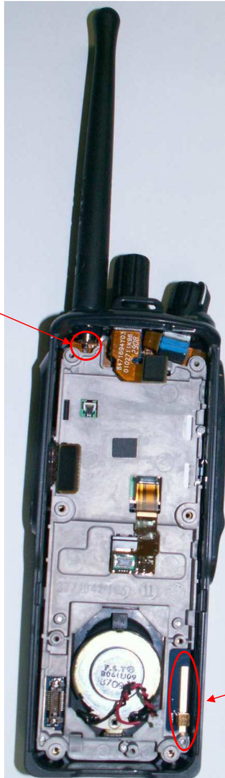
Photograph 9-7: View from back, main board removed, uncovering internal chassis. BT antenna visible at bottom right.
