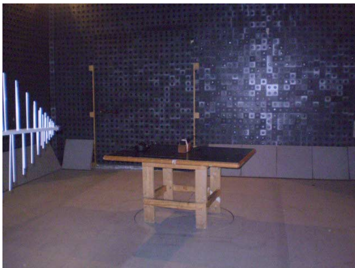
Photograph 7.2.1 Setup for carrier field strength measurements
