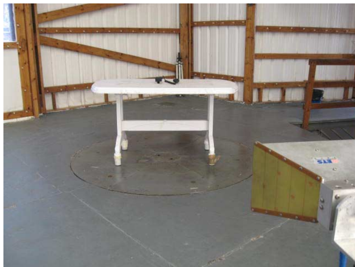
Photograph 7.1.4 Setup for spurious emission field strength measurements above 1000 MHz
