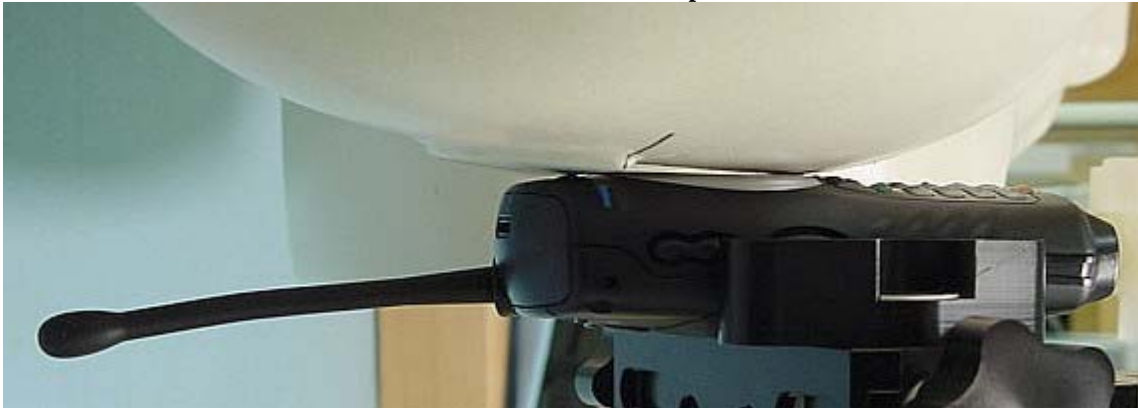
Figure 5. Assessment @ the Right ear. DUT in cheek touch position.
