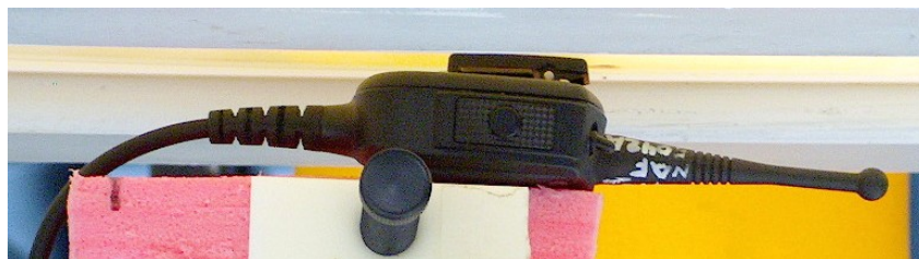
Figure 12: Body Assessment Public Safety Microphone (PSM) RMN5072A and antenna NAF5042AR against the phantom; (Same test position for other PSMs)
