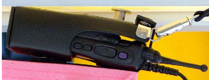
Figure 9: Body Assessment DUT w/ audio cable RMN4049A, carry strap NTN5243A, and NNTN4116A carry case, w/o swivel; back side of the carry case against the phantom.
