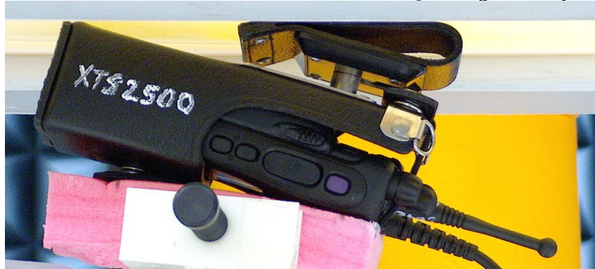
Figure 4: Body Assessment DUT w/ audio cable NMN6191C, and NNTN4115A carry case against the phantom.
