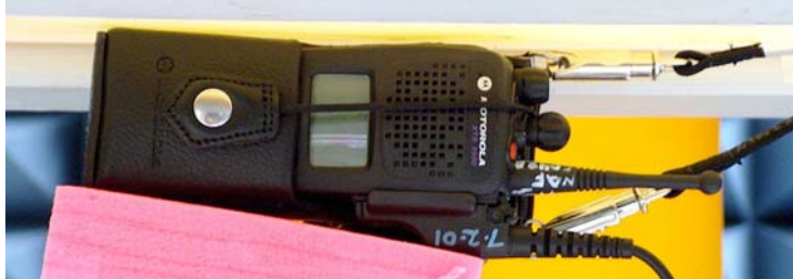
Figure 12: Body Assessment Public Safety Microphone (PSM) RMN5072A and antenna NAF5042AR against the phantom; (Same test position for other PSMs)
