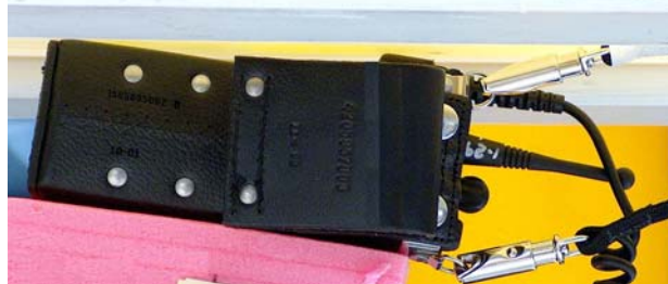
Figure 10: Body Assessment DUT w/ audio cable RMN4049A, carry strap NTN5243A, and NNTN4116A carry case, w/o swivel; right side of the carry case against the phantom. (Same test position for carry case NNTN4117A w/ carry strap NTN5243A)
