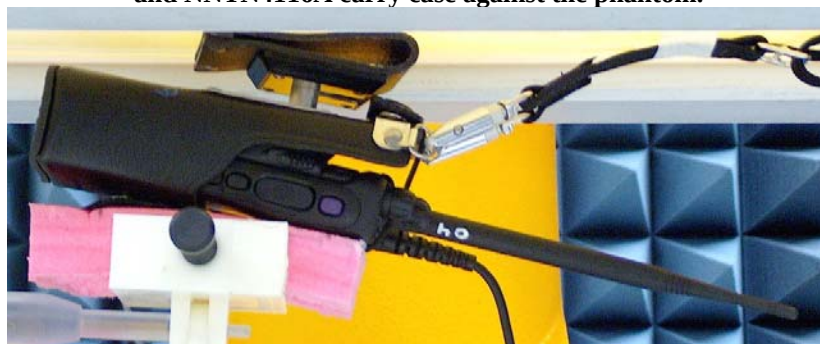
Figure 5: Body Assessment DUT w/ audio cable NMN6191C, carry strap NTN5243A, and NNTN4116A carry case against the phantom.
