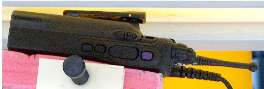
Figure 3: Body Assessment DUT w/ audio cable RMN4049A, and HLN9844A belt clip against the phantom.
