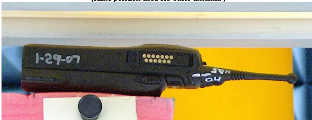
Figure 2: Highest SAR Test Position (face) DUT w/ front side separated 2.5cm from the phantom (same position used for other antenna )
