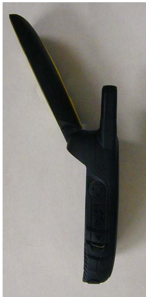
Figure 3-7. Side of i580 radio, flip open and Antenna retracted.
