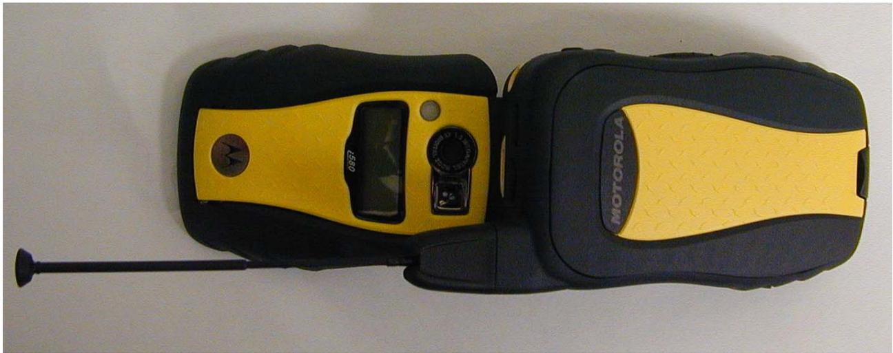
Figure 3-5. Back of i580 radio, flip open and antenna extended.
