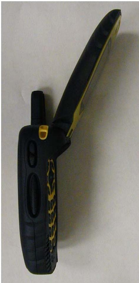
Figure 3-6. Side of i580 radio, flip open and Antenna retracted.
