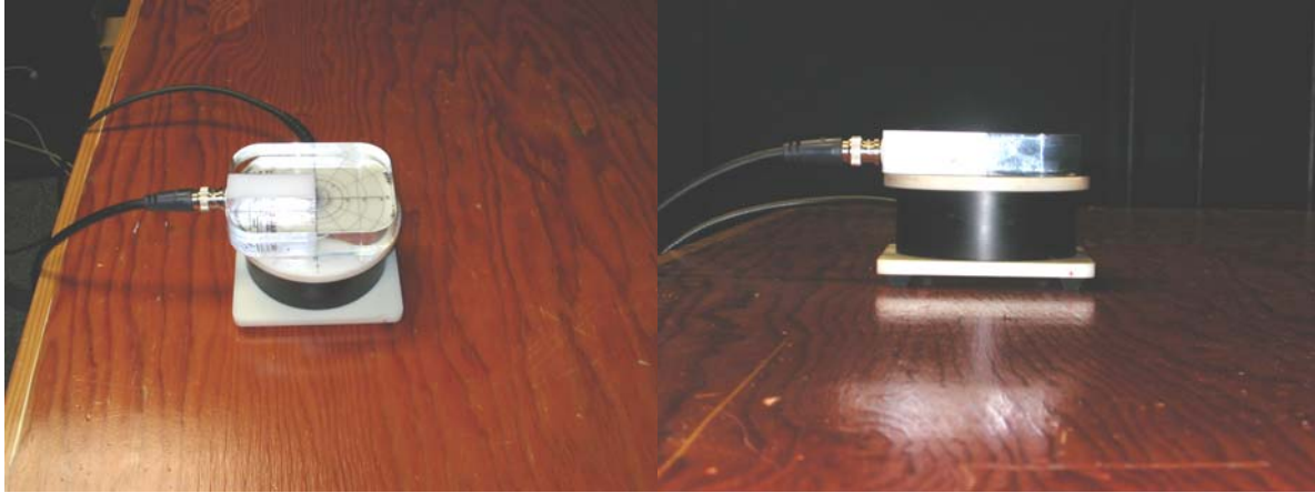
Figure 4 – Probe coil being calibrated with TMFS
