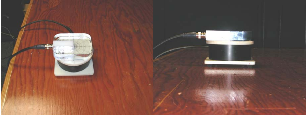
Figure 4 – Probe coil being calibrated with TMFS
