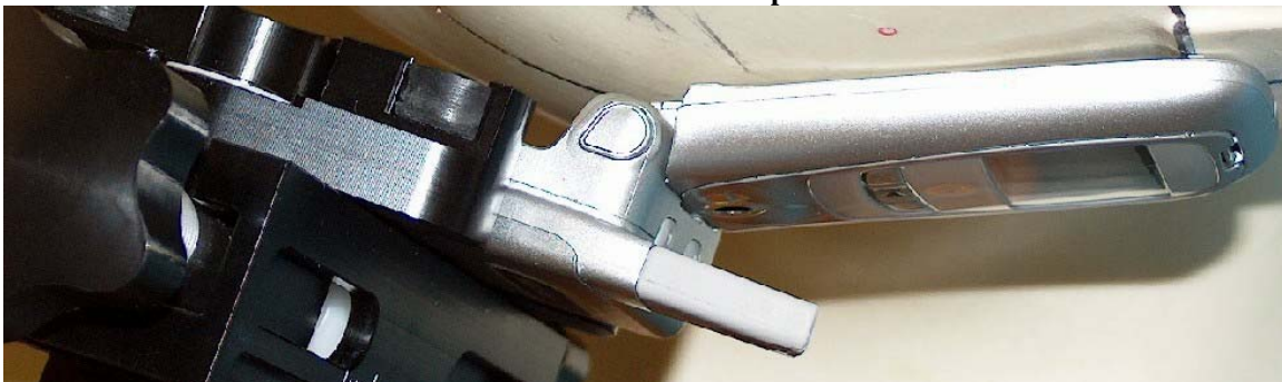
Figure 6: Head Assessment DUT at the left ear in touch position.
