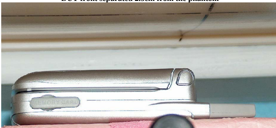
Figure 9: Body Assessment DUT front separated 2.5cm from the phantom
