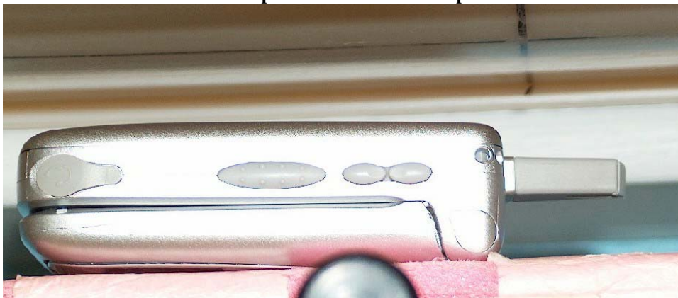
Figure 9: Body Assessment DUT front separated 2.5cm from the phantom
