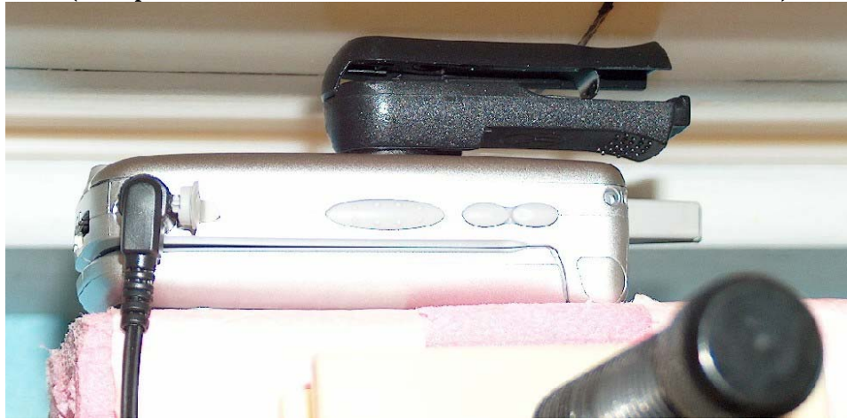
Figure 4: Body Assessment DUT with carry accessory model NNTN4747A against the phantom. (same position used for each attached data and audio cable accessories)
