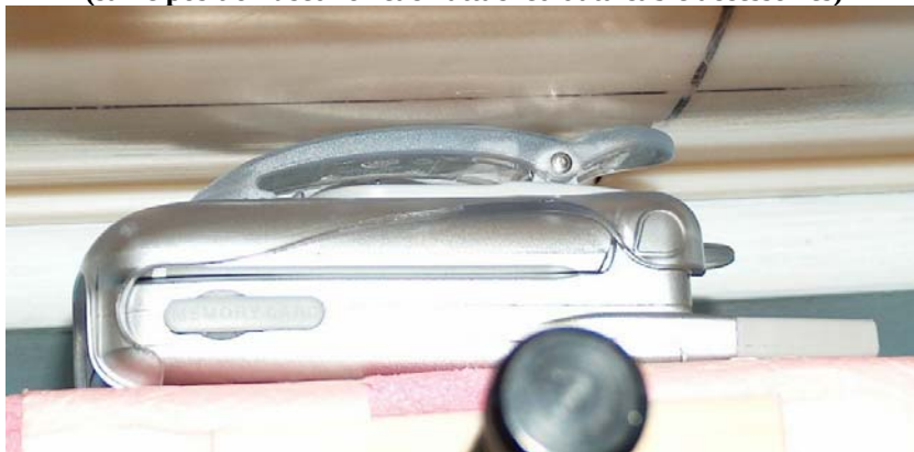
Figure 3: Highest S.A.R. Test Position (Body) DUT with carry accessory model NNTN6231A against the phantom. (same position used for each attached data cable accessories)
