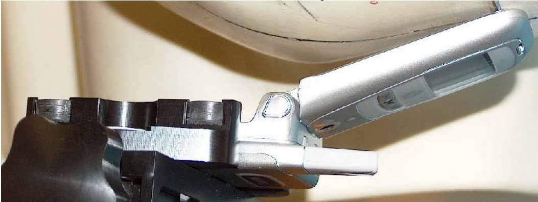
Figure 8: Body Assessment DUT back separated 2.5cm from the phantom
