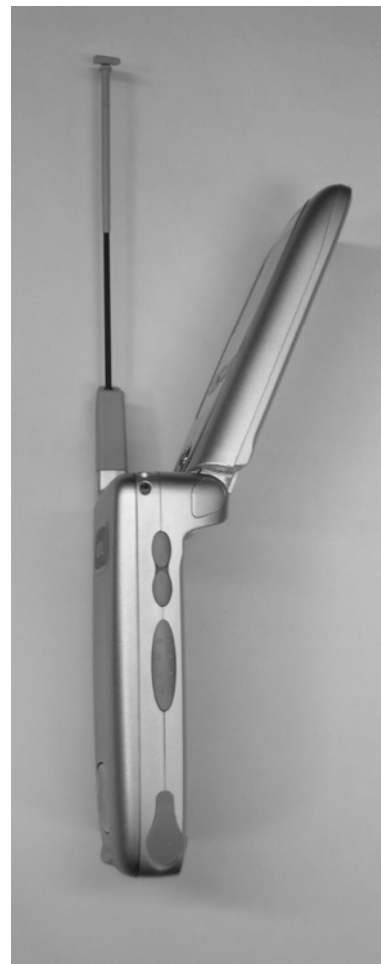
Figure 3-9. Side of i870 radio, flip open and antenna extended.
