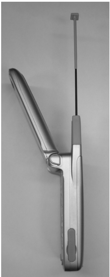
Figure 3-8. Side of i870 radio, flip open and antenna extended.
