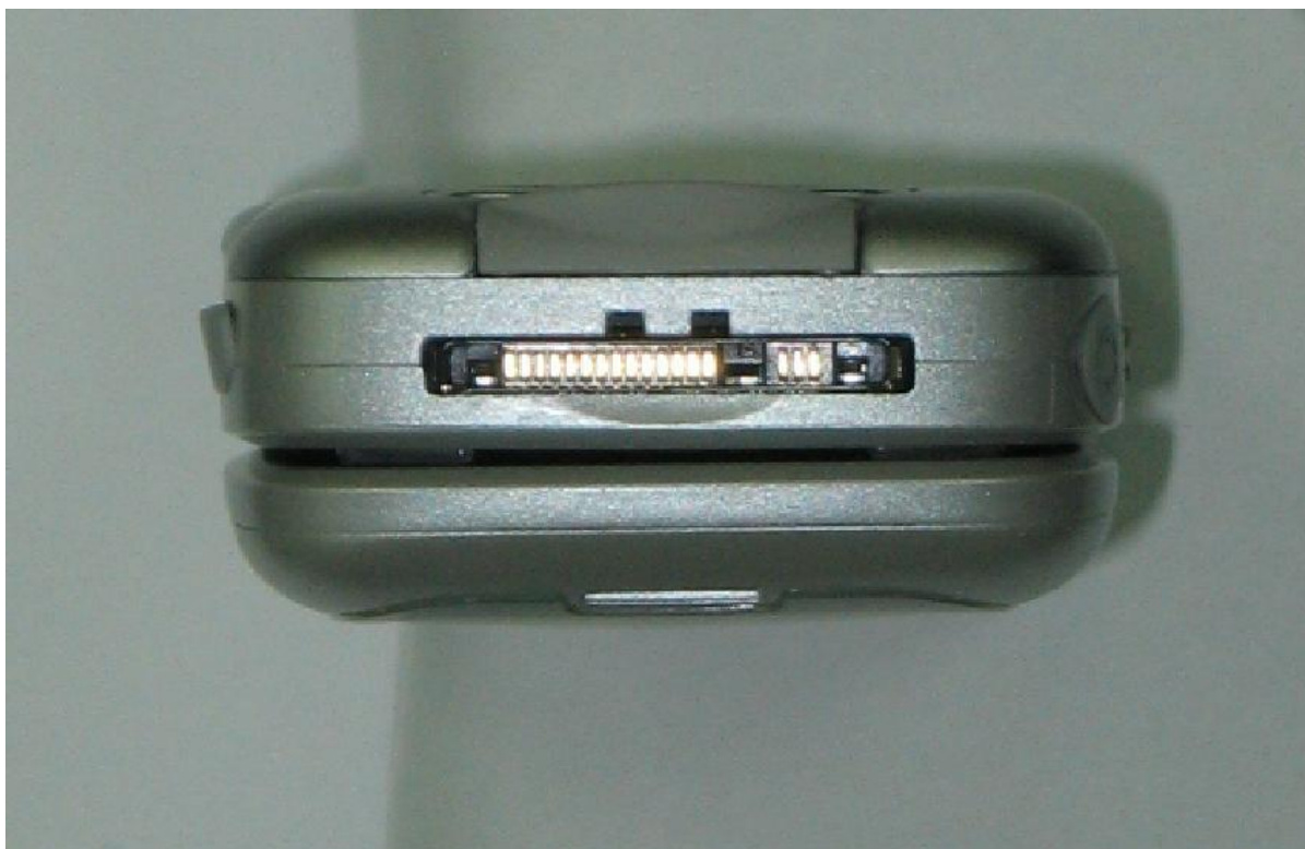
Figure 3-13. Connector end of i870 radio.
