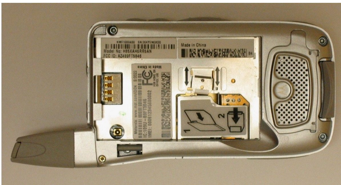
Figure 3-14. Battery Compartment of i870 radio.
